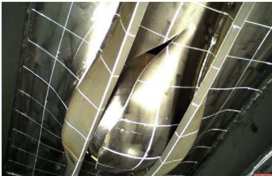
> Figure 3-2 Experimental test. Indentation of panel with 2 HP-stiffeners [17].
