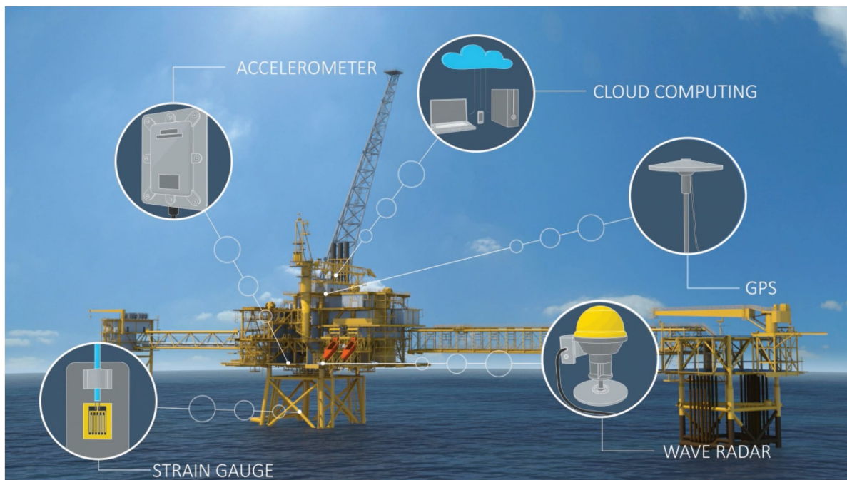
Figure 5-1: An example of measurement equipment and sensor technology for data collection.
