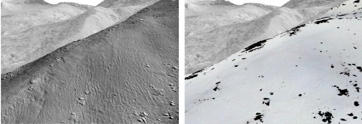
**Figure 5.8 Shaded relief with 10 cm resolution generated from lidar point cloud (left) compared to an orthophoto (right), from the same snow accumulation zone.**
