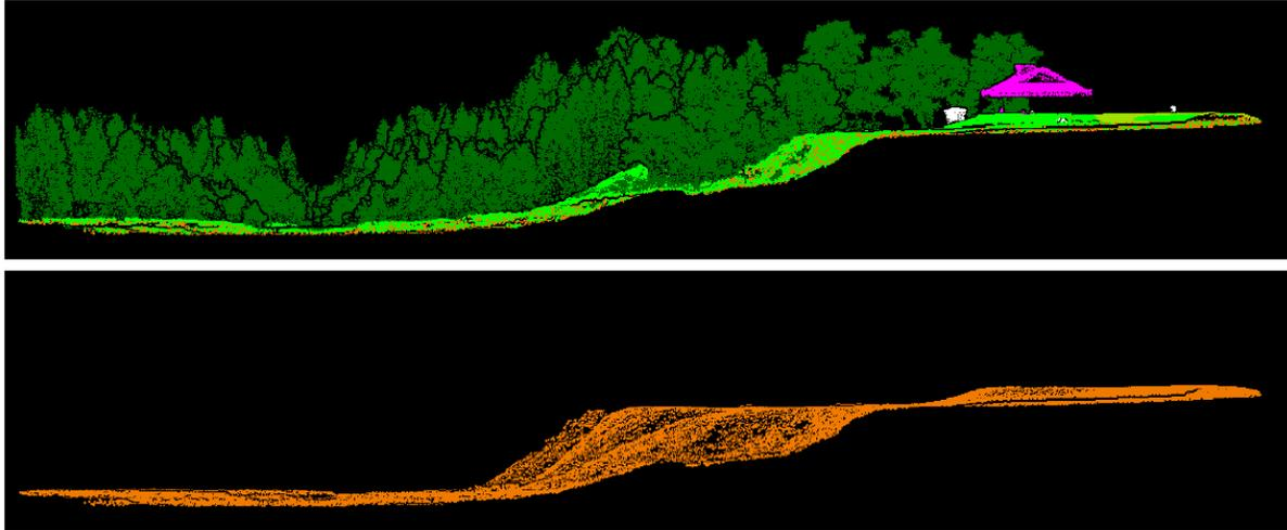
**Figure 4.9** Output from KVS of site A showing point cloud and the terrain only.
