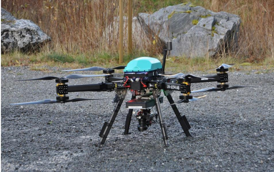
**Figure 4.7 KVS Quadcopter with Lidar Sensor.**
