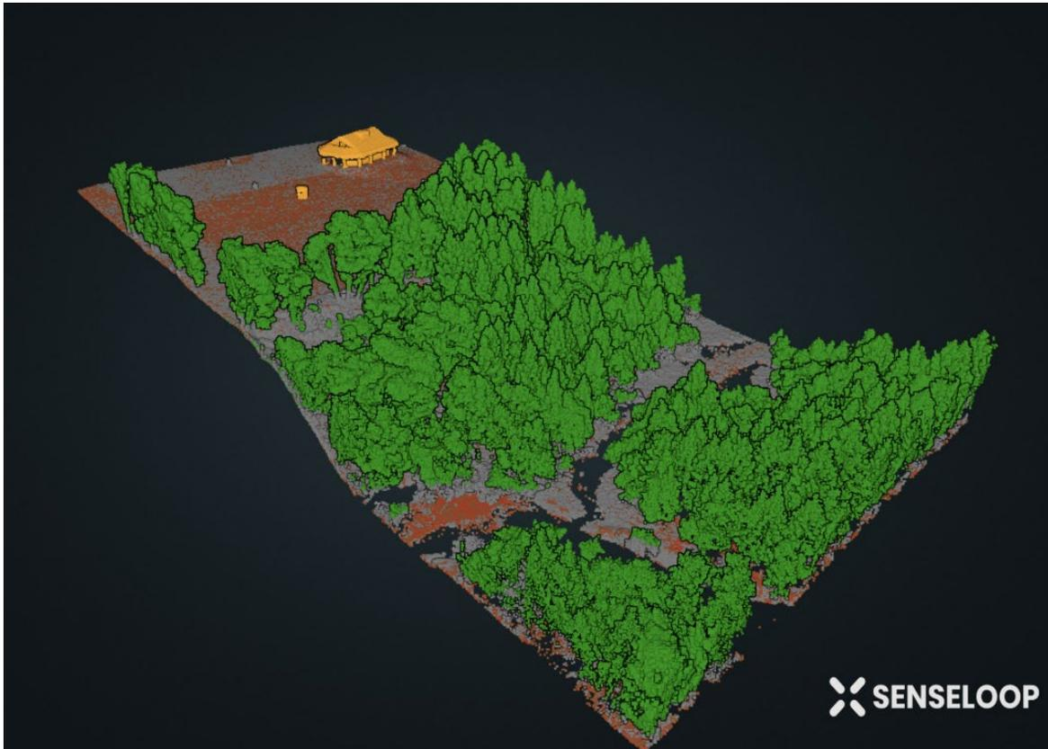
Figure 4.13 Classified point cloud of site A provided by Senseloop.
