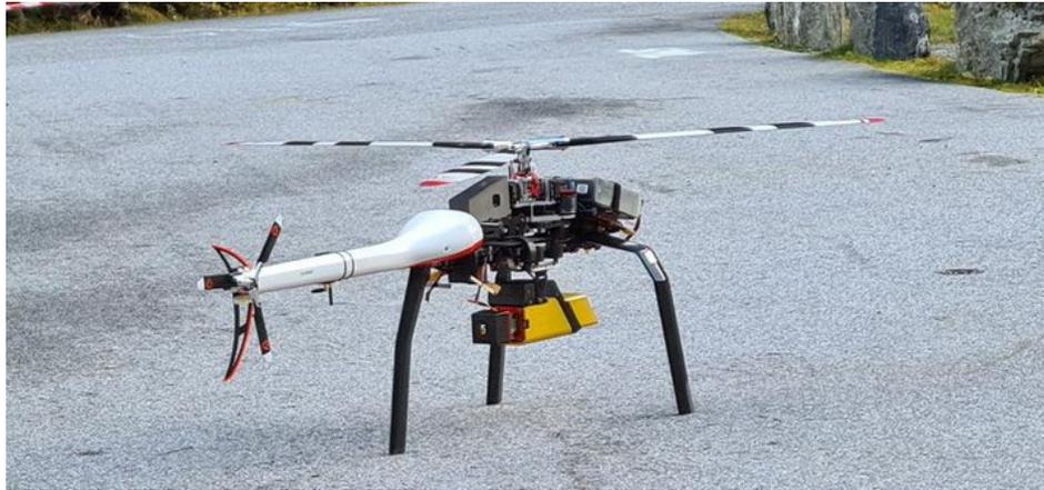
**Figure 4.16 Velos Helicopter with Lidar Scanner.**
