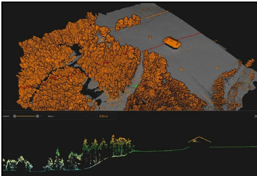
**Figure 4.17 Classified point cloud and section profile from Site A provided by Orbiton.**
