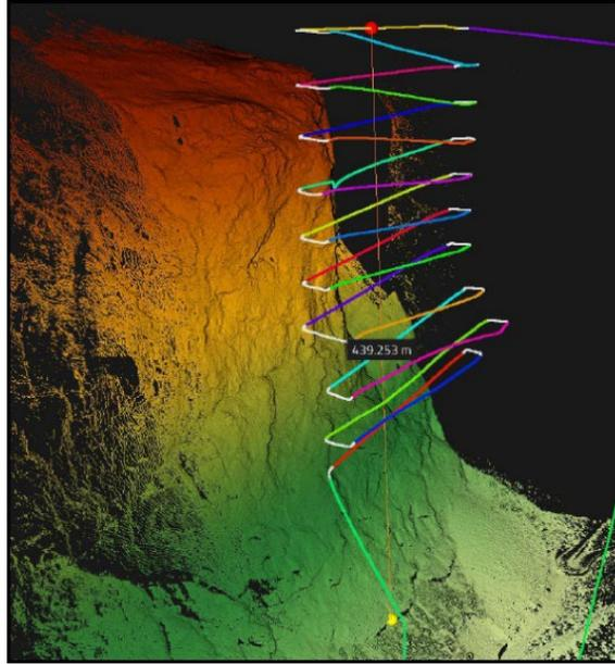
**Figure 4.18 Flight path and Lidar point cloud colored by elevation from Site B provided by Orbiton.**
