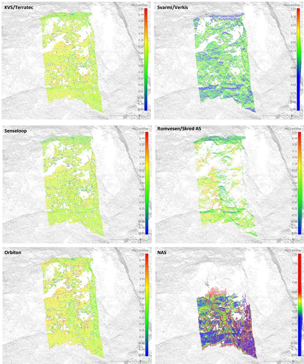
**Figure 5.3 Three-dimensional cloud-to-cloud distance (m) between acquired point clouds and the National Elevation Model (NDH). Distances are calculated with M3C2 plugin in CloudCompare and represent the distance between nearest neighbors along surface normal vectors (15). The color range stretches from < -0.5 m (blue) to > 0.5 m (red). Point cloud from the NDH is shown in grey.**
