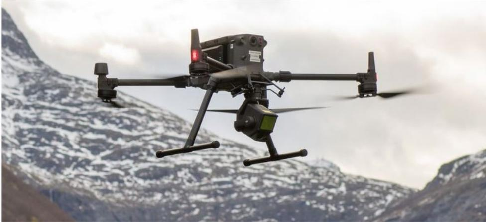
**Figure 4.20 NPRA drone, DJI M300. (Photo: Ove Kristian Leirgulen)**
