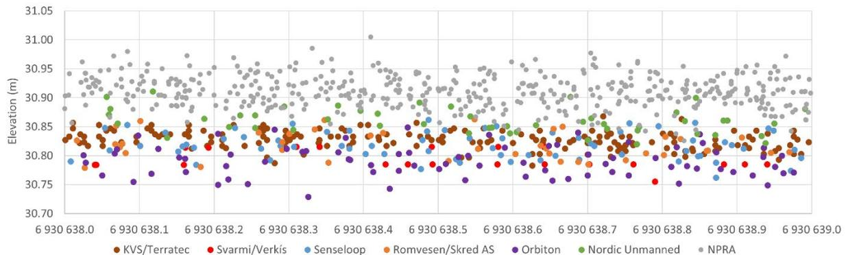
**Figure 5.1 Small-scale point cloud precision illustrated by points collected in a 1 x 0.2 m nearly flat region covered by compacted gravel. The surface roughness of the gravel is estimated to be around 1–2 cm.**
