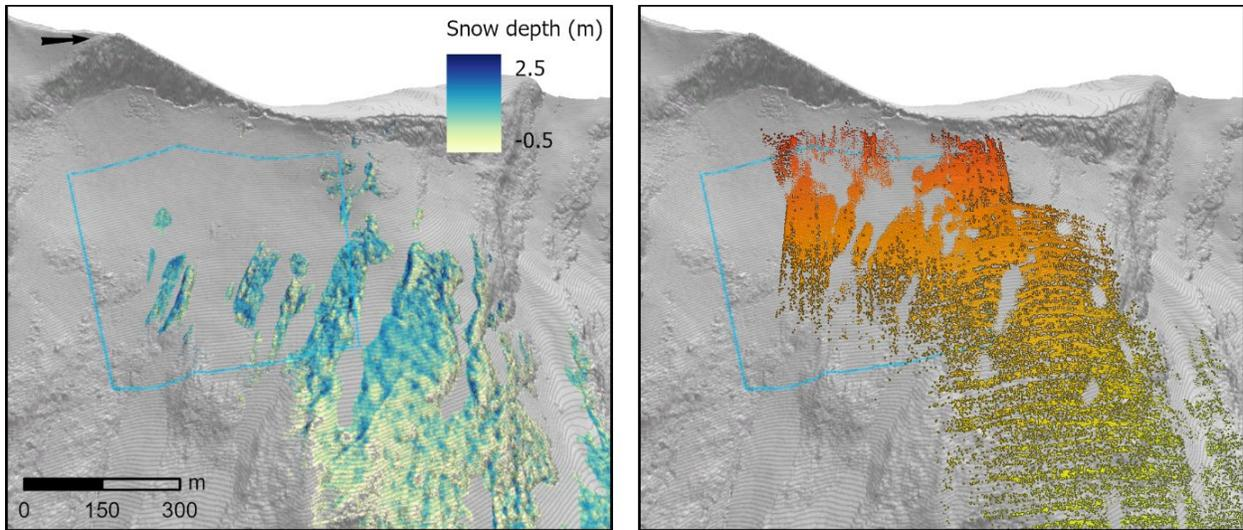
**Figure 5.9 3D view of snow depths (left) and coverage (right) of lidar data from Orbiton at site C2.**
