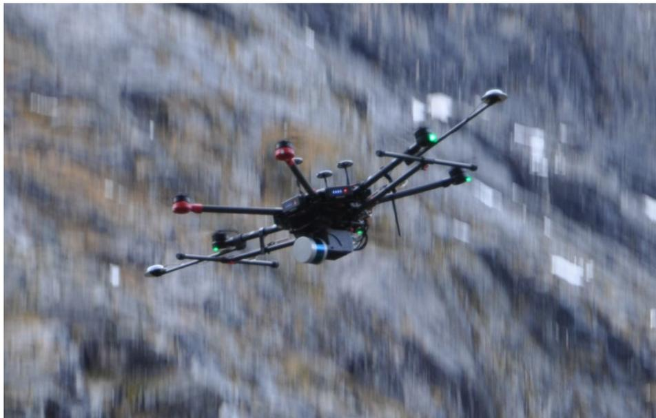
**Figure 4.19 Norse Asset Solution's DJI M600 with Velodyne Ultra Puck lidar.**
