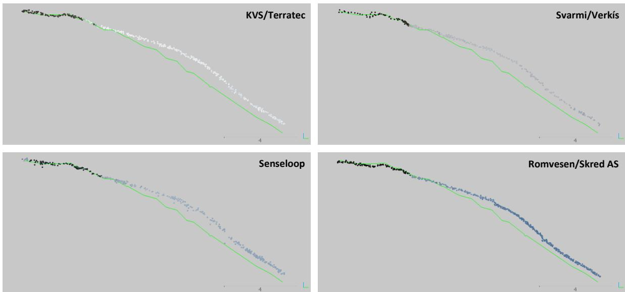
**Figure 5.7 Point cloud sections from bare ground into a snow accumulation zone. The points are gathered along the blue line shown in the right image, within a width of 20 cm and from all point classes. The green reference line represents a rough approximation of the snow-free ground interpolated from classified ground points in the NDH point cloud.**
