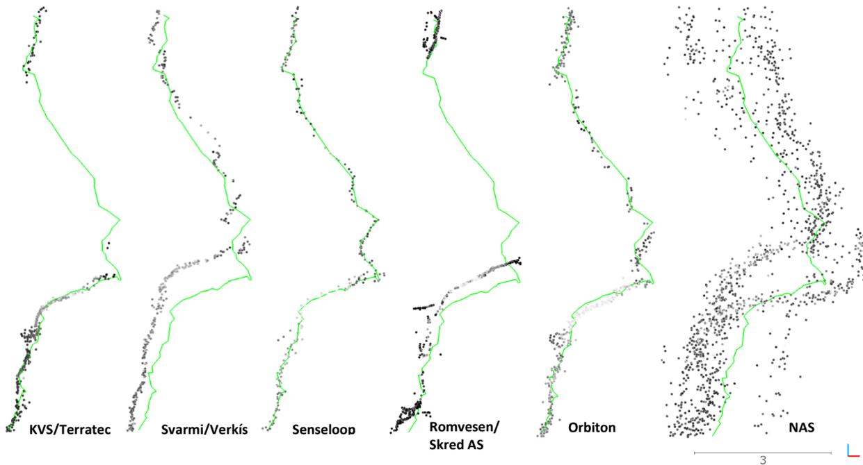
**Figure 5.4 Point cloud sections across an overhanging part of the rock wall. The green line represents a reference surface interpolated from Senseloop’s point cloud. Their point cloud shows good coverage in steep areas and good agreement with the National Elevation Model.**
