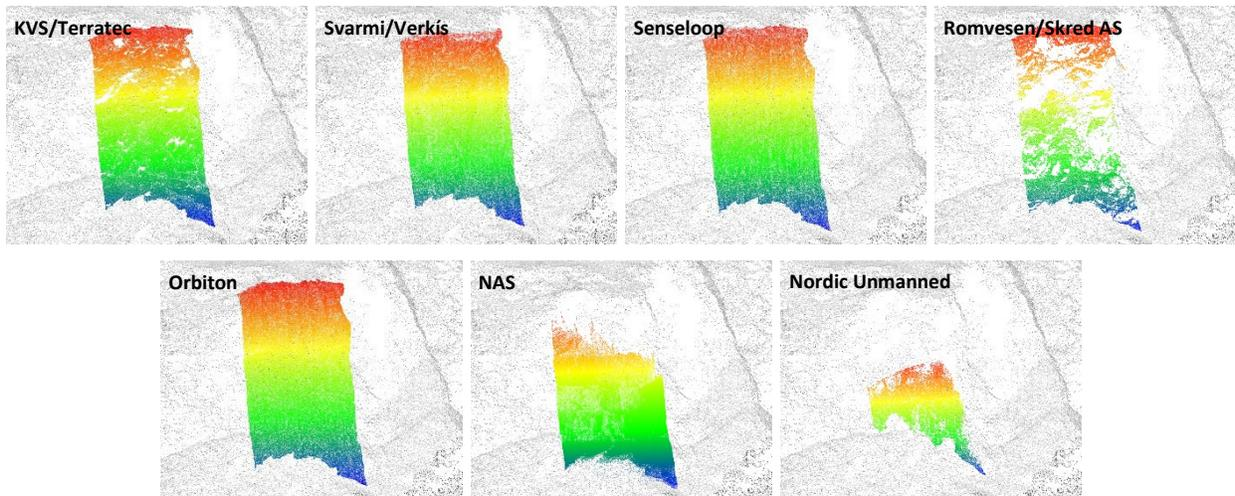
**Figure 5.2 Area coverage at site B shown by colored points from within the specified survey area. Point cloud from the National Elevation Model (NDH) from the Norwegian Mapping Authority is shown in grey.**
