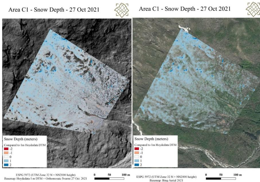
**Figure 4.12 Snow depth map (Svarmi Lidar minus Hoydedata 1 m DTM) provided by Svarmi/Verkís.**
