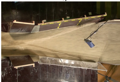
Skred 29: B = 300 \text{ mm} , \beta = 10^\circ
