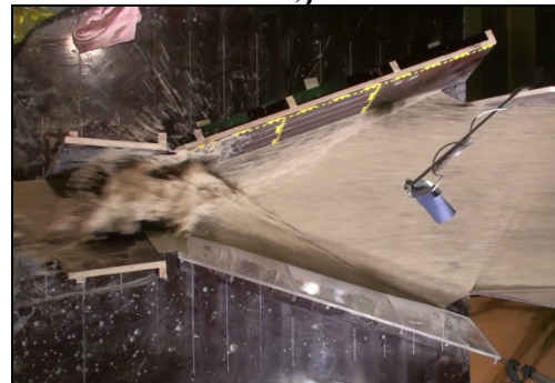
Skred 43: B = 100 \text{ mm} , \beta = 20^\circ
