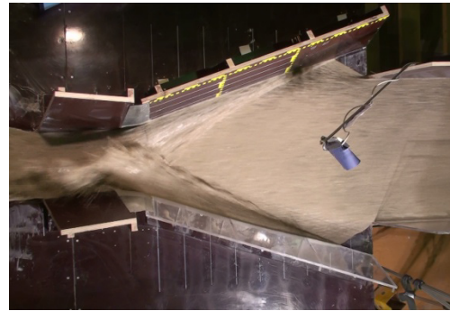
Skred 38: B = 200 \text{ mm} , \beta = 20^\circ
