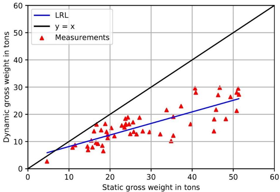
*Figure 28 Static / raw and calibrated dynamic gross weights Losna E6*
