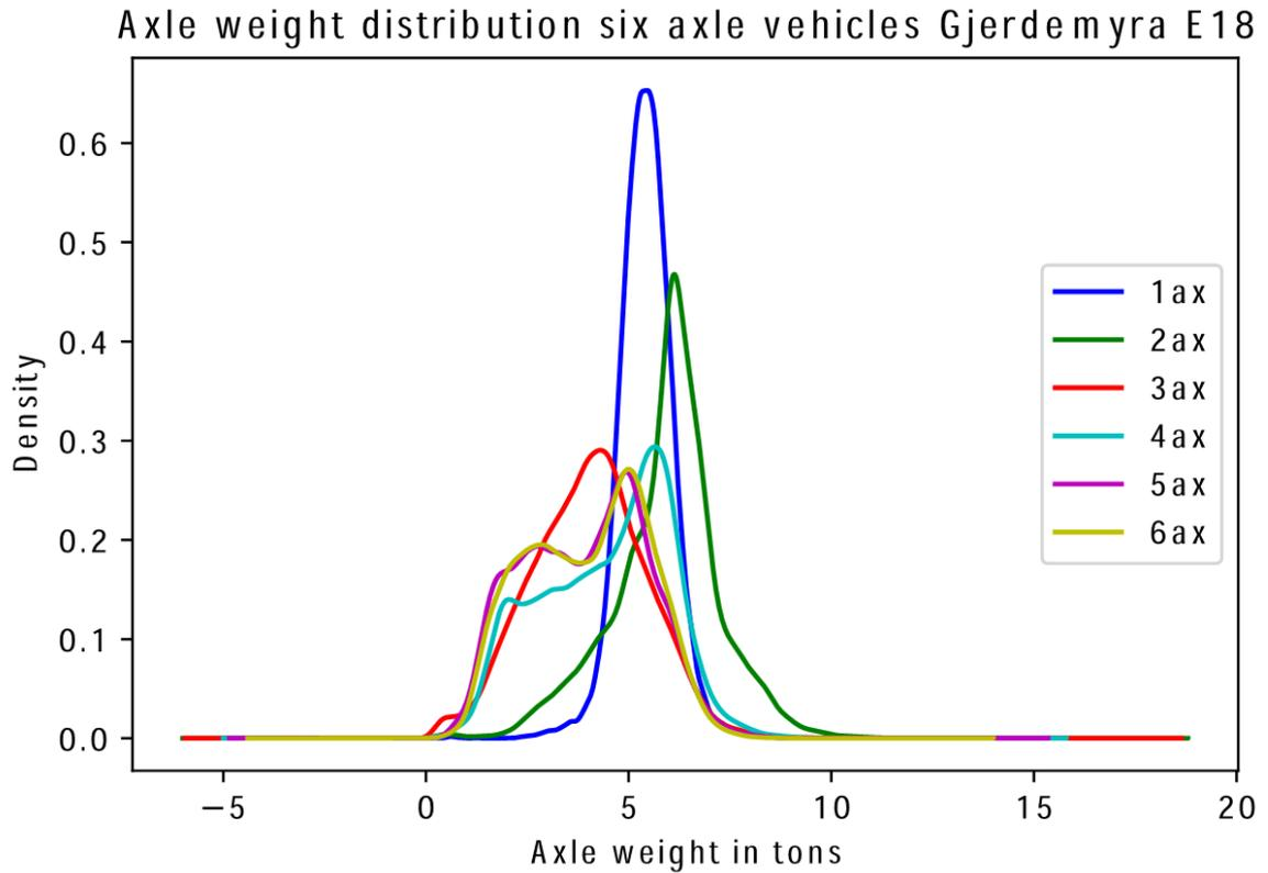
Figure 12 KDE plot raw axle weight data 6 axle vehicles Gjerdemyra E18
