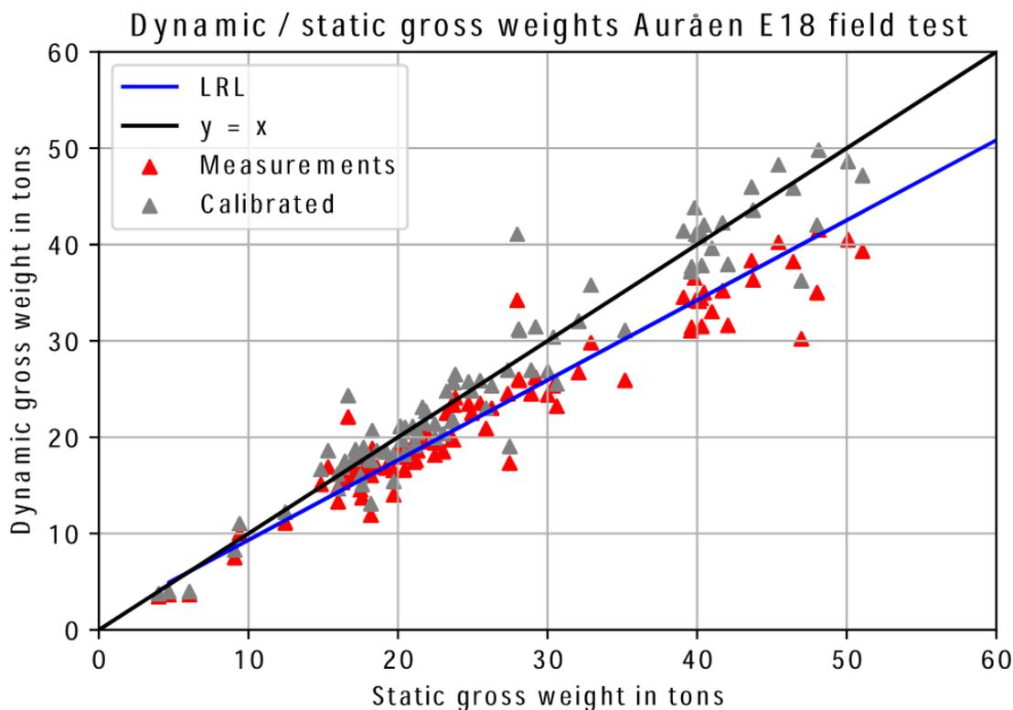
Figure 26 Static / raw and calibrated dynamic gross weights Auråen E18
