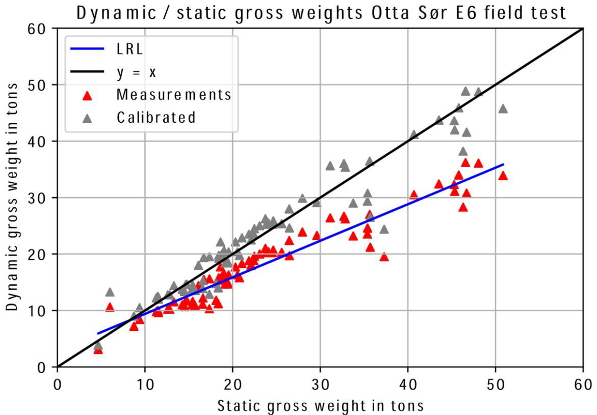
Figure 18 Static / raw and calibrated dynamic gross weights Otta E6
