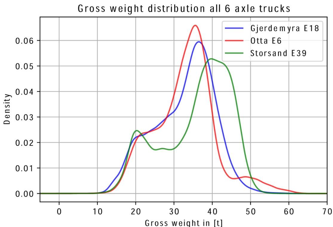
Figure 7 Gross weight distribution of six axle trucks at ATK points Gjerdemyra, Otta and Storsand
