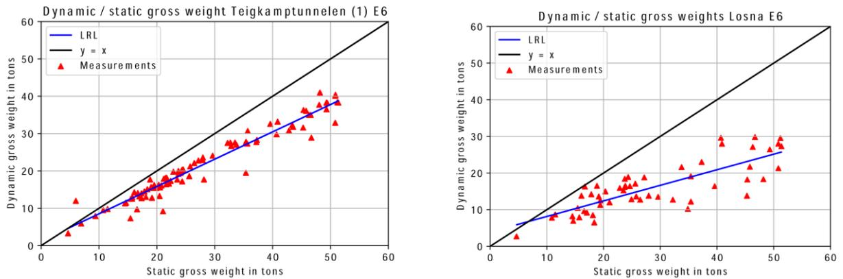
Figure 6 Field test results for ATK points Teigkamptunnelen and Losna along E6 in Oppland 2016
