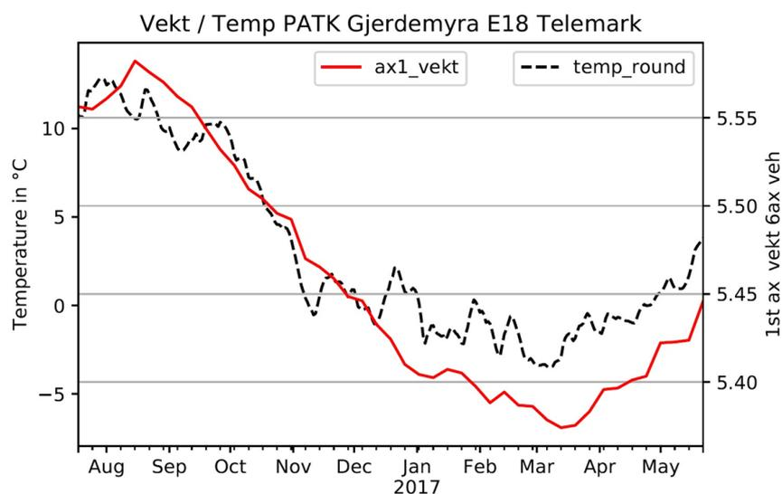
Figure 8 Temperature impact on ATK raw data accuracy [local air temperature compared to weight of first axle of six axle semi-trailer vehicles]
