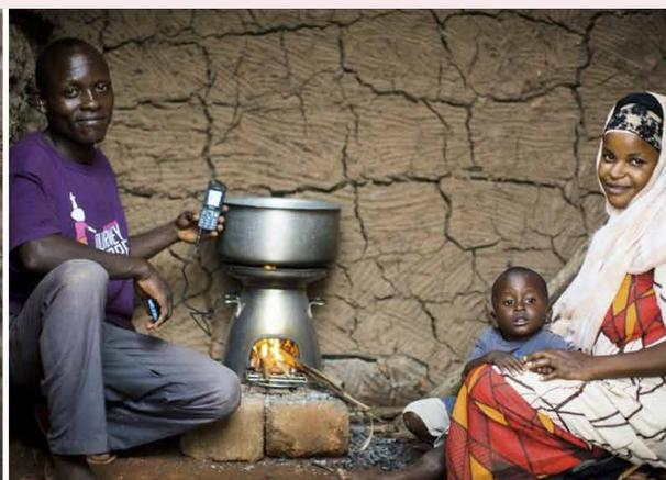
A relatively advanced cook stove where the heat from the flame is converted into electricity through a thermoelectric generator. This electricity powers an internal fan, which force-feeds oxygen into the flame, eliminating the smoke, and leading to the near complete and clean combustion of the fuel. The stove generates surplus electricity – enough to charge a mobile phone and provide an evening's worth of LED
