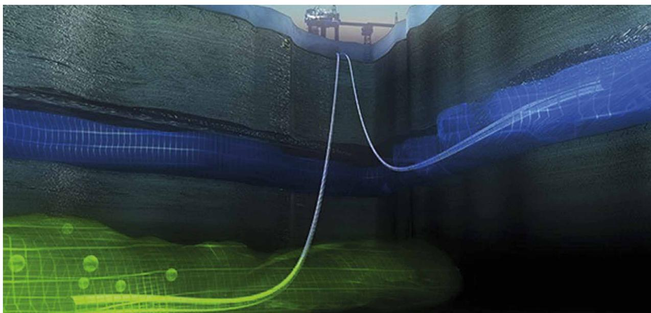
Picture: Illustration of CO<sub>2</sub> injection and storage on the Sleipner field in the North Sea. The gas from the field has a high content of CO<sub>2</sub>. During processing of the gas on the platform, CO<sub>2</sub> is separated and injected into the Utsira formation far below the seabed. Since 1996, up to 1 million tonnes of CO<sub>2</sub> a year has been stored here. Statoil is the operator for Sleipner (Photo: Alligator film/BUG, Statoil).
