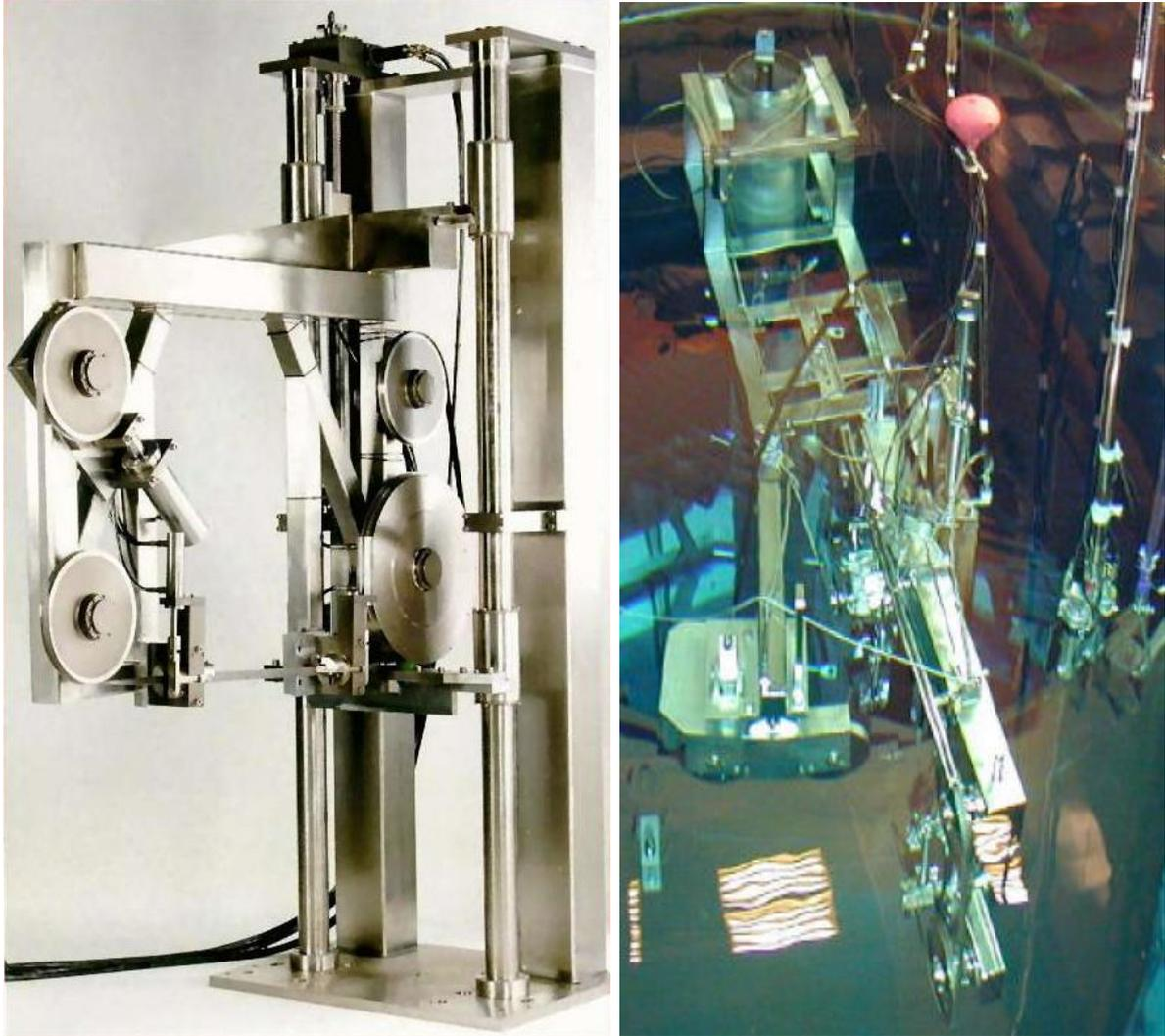
*Figure 5. Manufacturers photograph of the BR-3 Band Saw (left) and the Forsmark Band Saw being used to segment the Core Shroud (or Moderator Tank).*
