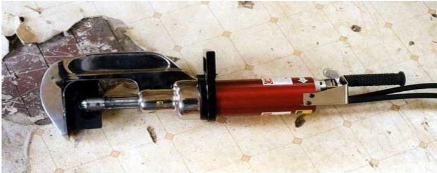
*Figure 13. Mega-Tech Services Inc. Blade Plunging Cutter.*
