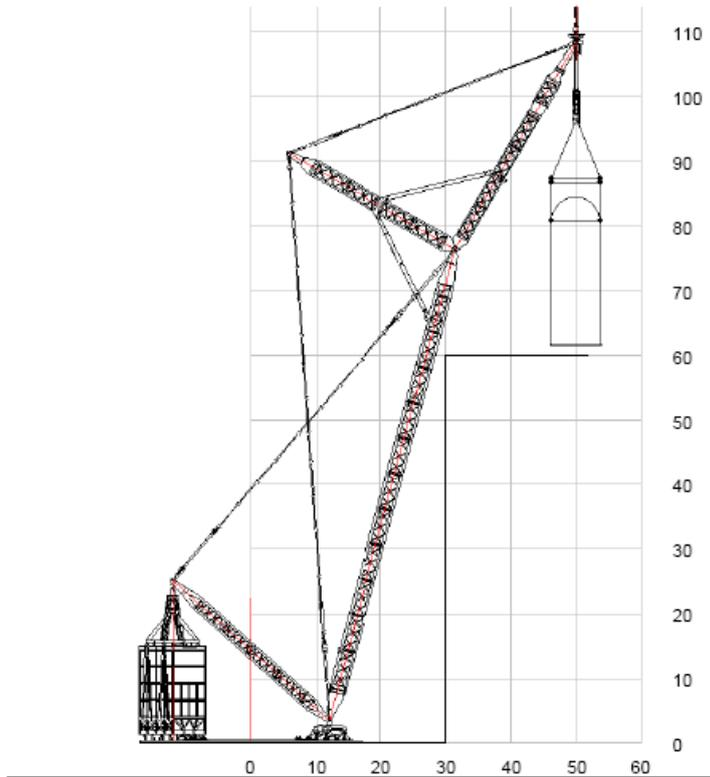
Figure 8. Lift of a RPV with a Mammoet MSG 80.
