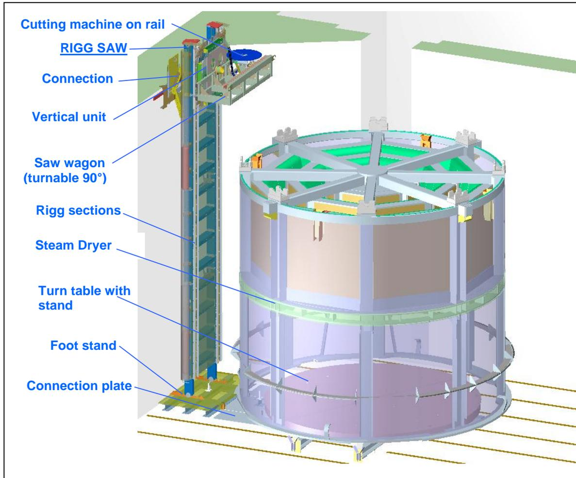
Figure 6. Rig saw with a disc saw mounted to cut the Steam Dryer.
