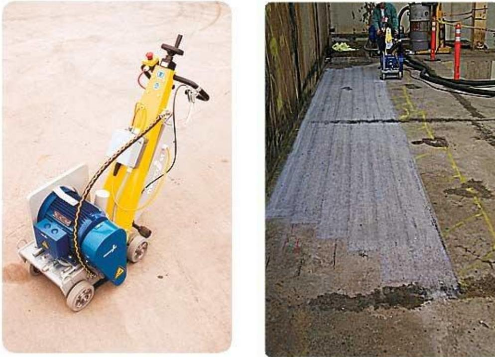
*Figure 17. Marcryst Floor Shaver and the resulting floor surface.*
