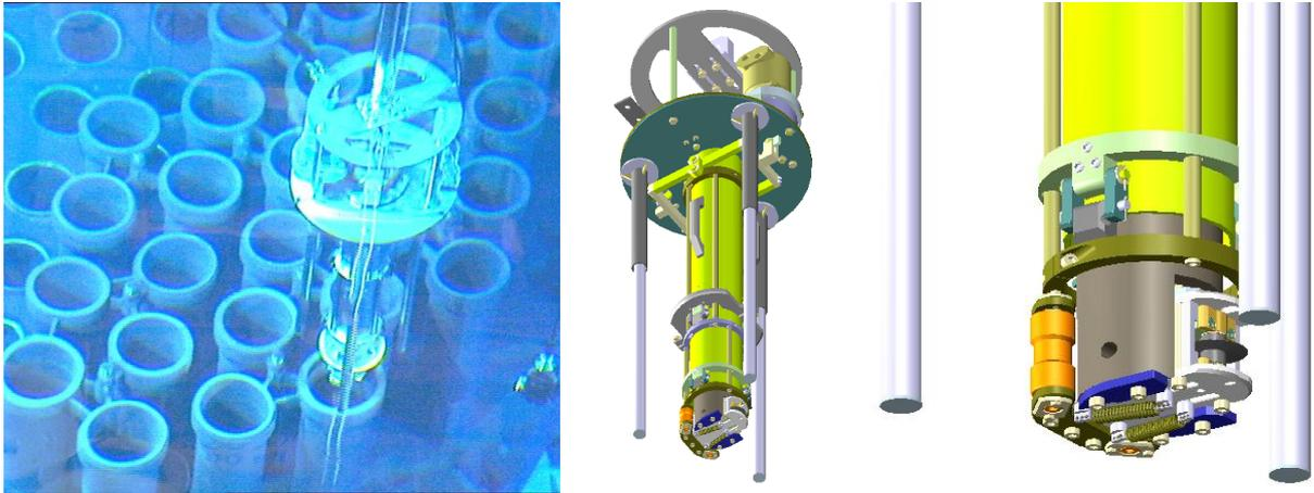
Figure 7. The tube cutter is positioned above the CSH piping. 3D-model views of the tube Cutter.
