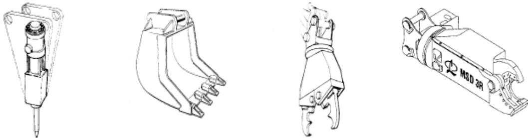
Figure 22. Examples of tools for use with demolition machines.
