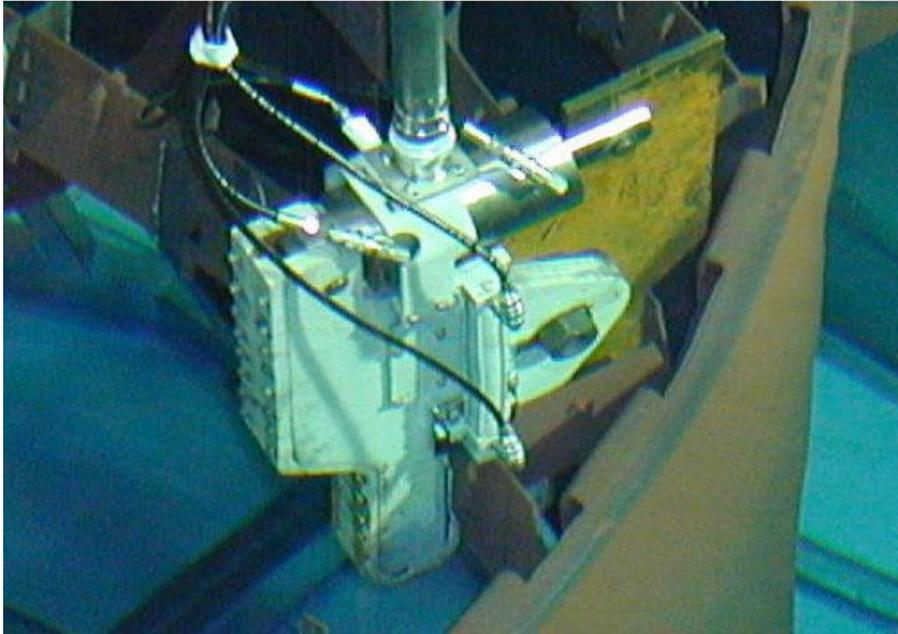
*Figure 4. Hydraulic Shears being used for cutting of the Core Grid removed from the Forsmark Nuclear Power Plant.*
