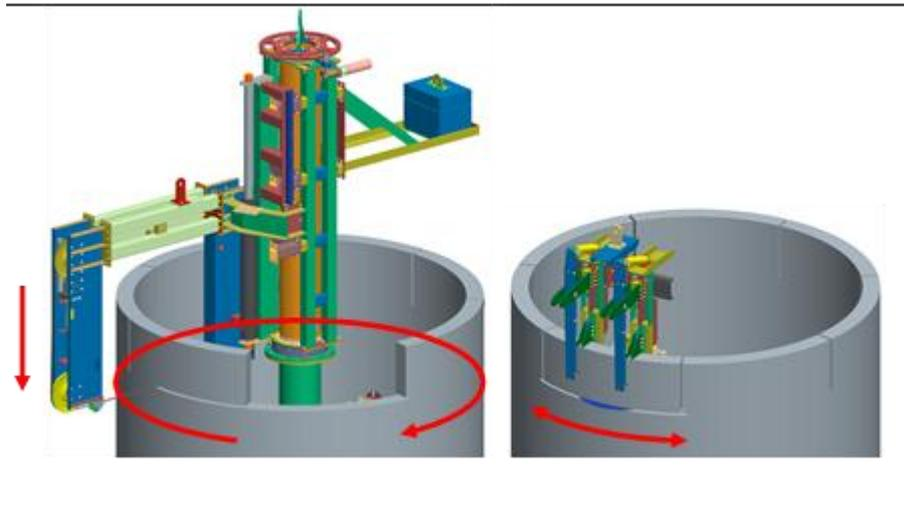
Figure 9. Model of the mechanical cutting of the RPV at José Cabrera.
