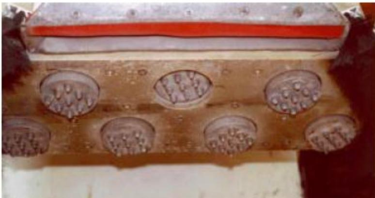
Figure 16. View of underside of PENTEK Moose cutting head.
