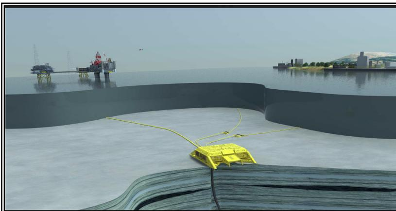
Figure 6-13: CO<sub>2</sub> injection well
