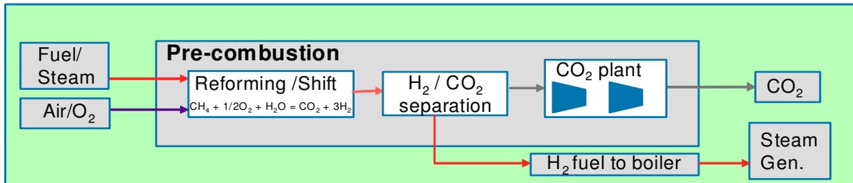
Figure 3-6 Pre-combustion steam generation
