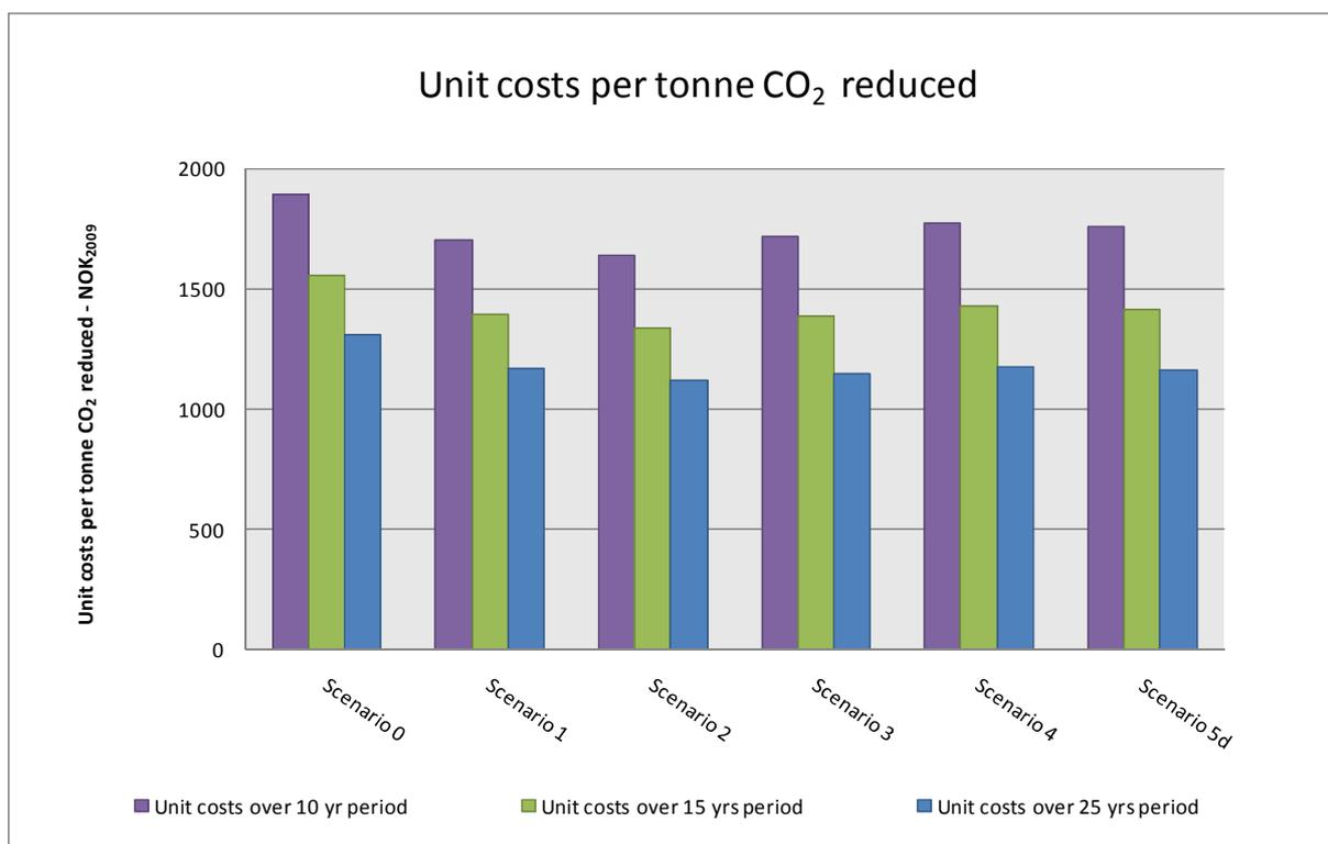
Figure 11-3 Total unit cost per tonne CO<sub>2</sub> reduction over 10, 15 and 25 years, exclusive of CO<sub>2</sub> quotas.
