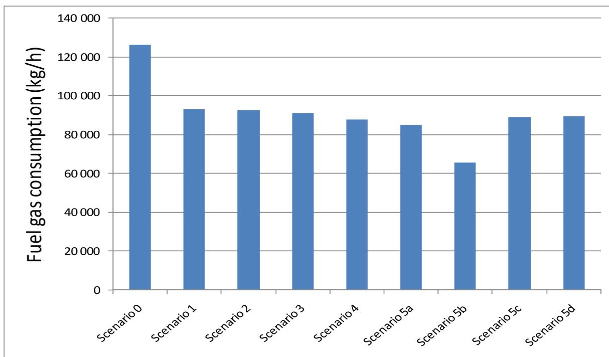
Figure 10-5 fuel gas consumption for the various scenarios
