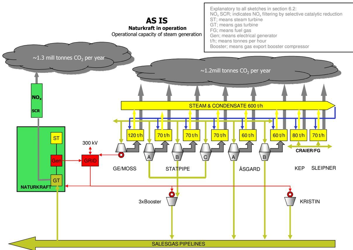
Figure 6-2 Schematic overview of existing facilities (As-is)
