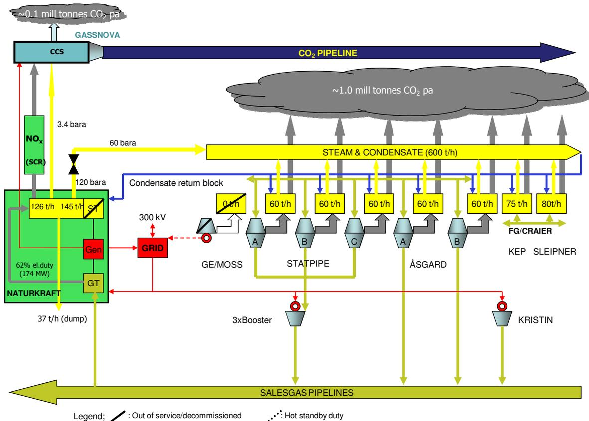
Figure 6-4 Schematic overview of scenario 1
