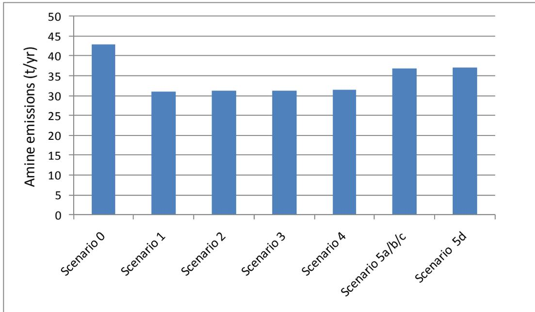
Figure 10-4: Estimated amine emissions from the carbon capture plant
