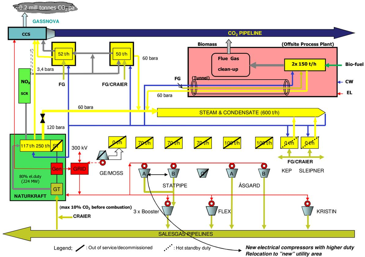
Figure 6-10 Schematic overview of scenario 5b
