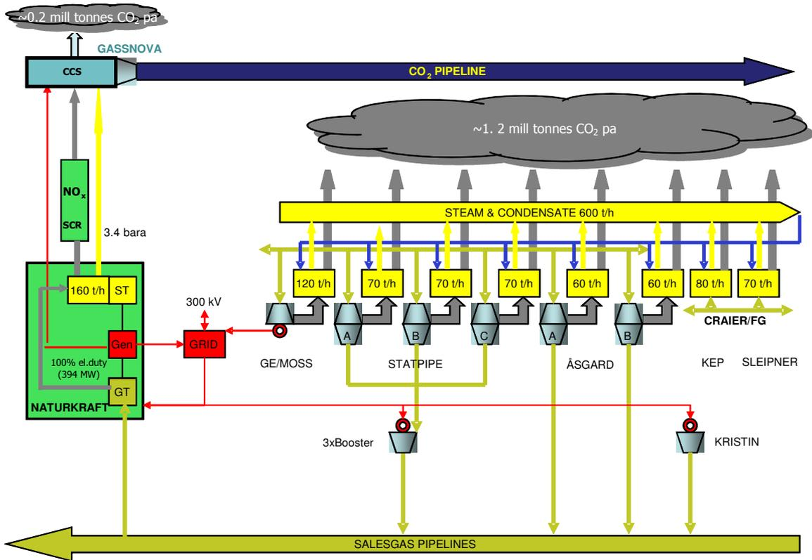
Figure 6-4 Schematic overview of scenario 0
