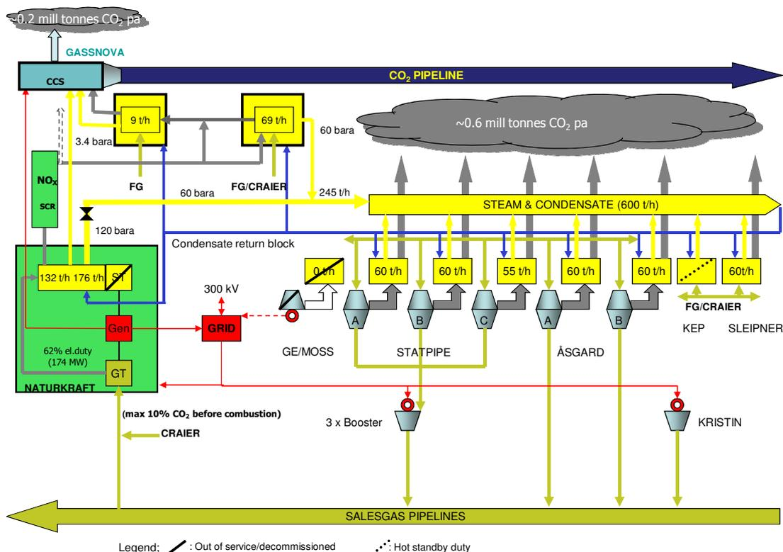
Figure 6-6 Schematic overview of scenario 3
