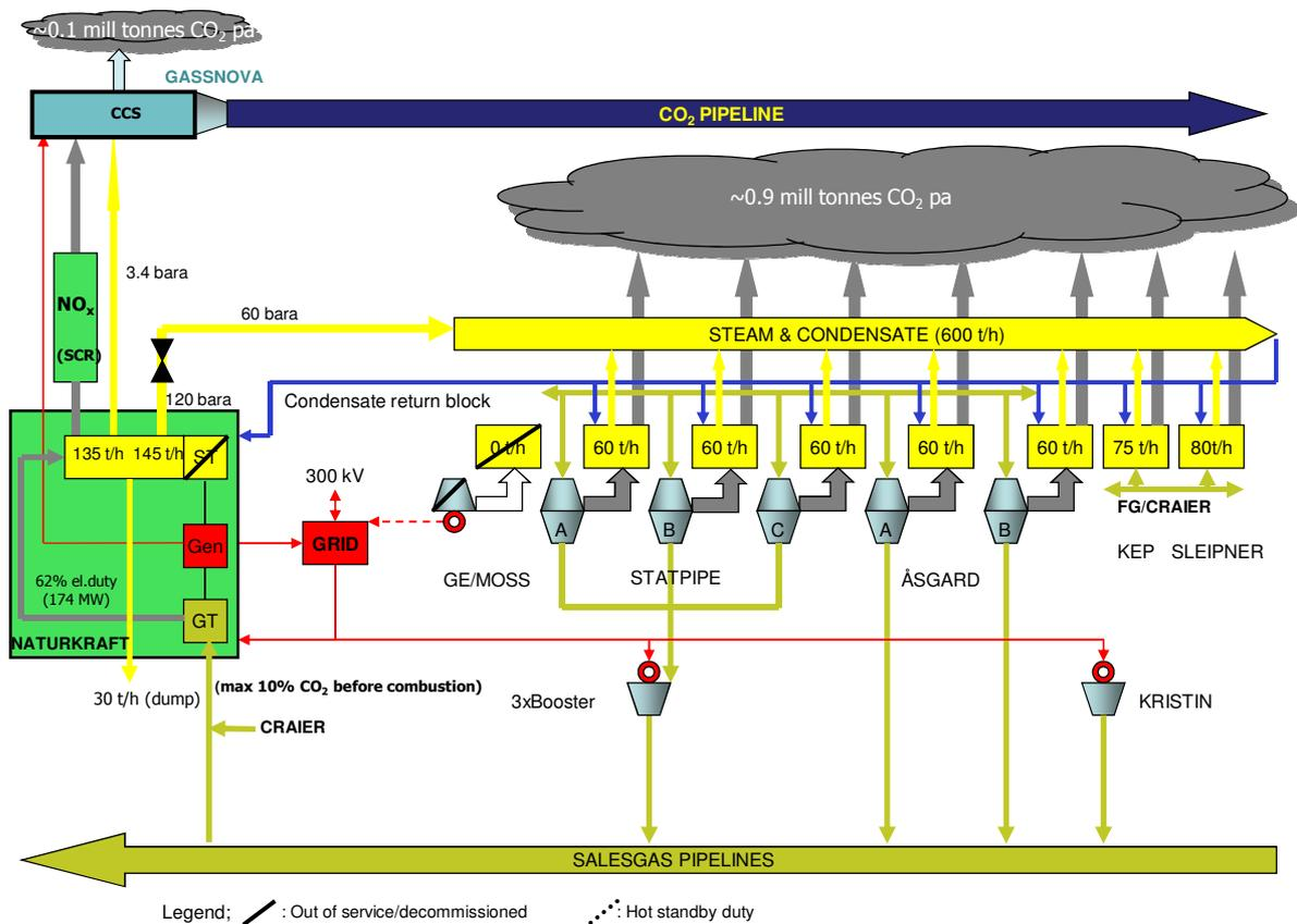
Figure 6-5 Schematic overview of scenario 2
