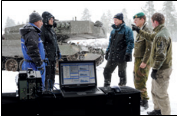
Figure 7.2 Noise level tests: Military activity can cause a high level of noise for its surroundings. The Norwegian Defence Research Establishment charts the noise levels generated by different types of weapon and vehicles, during varying weather conditions and seasons.
