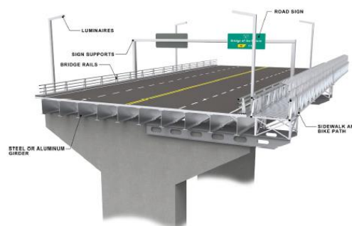
Figure 8. Use of aluminum in secondary bridge components.
