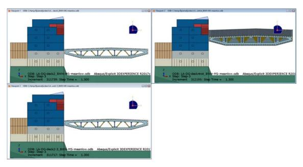
> Figure 5-1 Load cases A-C of deckhouse-girder collision side view: At deck 2 (upper left), inclined at deck 4 (upper right), between deck 2 and 3 (lower left)
