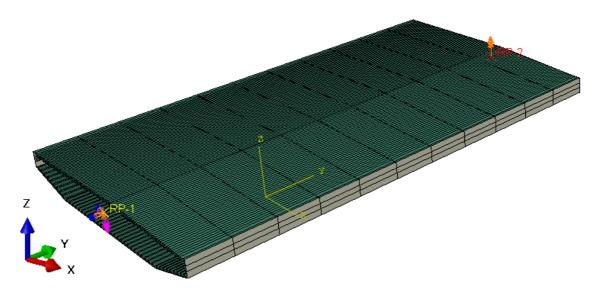
> Figure 4-14 Rotation about strong axis applied to the cut-off boundaries of the bridge girder
