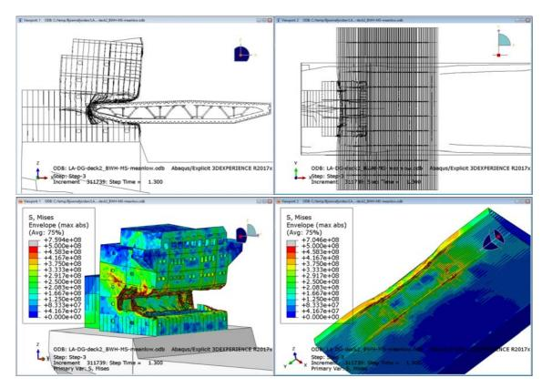
Figure 5-2 von Mises stress [MPa] load case A: Bridge girder at deck 2
