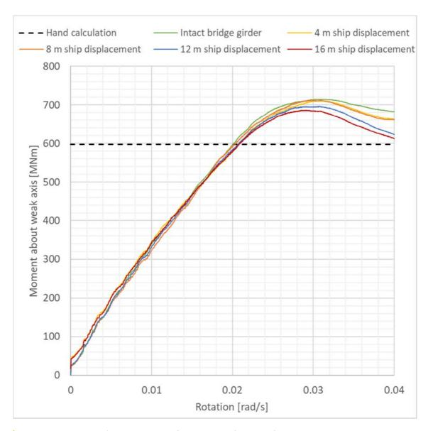
> Figure 5-14 Load-rotation curve for moment about weak axis
