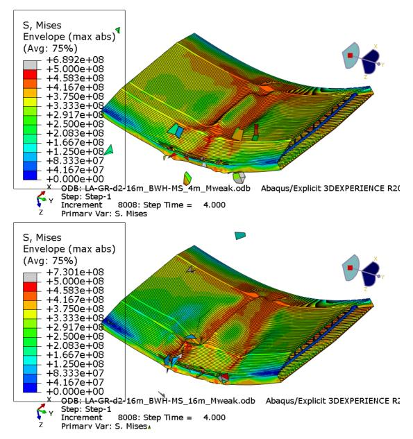
> Figure 5-12 Damaged bridge girder after 4 m (upper) and 16 m ship displacement (lower) applied with moment about weak axis. Deformations are scaled with factor 10 (and cause enlargement of damaged elements).
