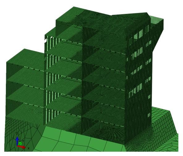
> Figure 4-7 Mesh of the deckhouse ship, shown cut in half
