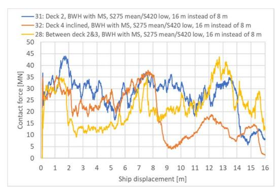
Figure 1 Contact force [MN] impact deckhouse-girder
