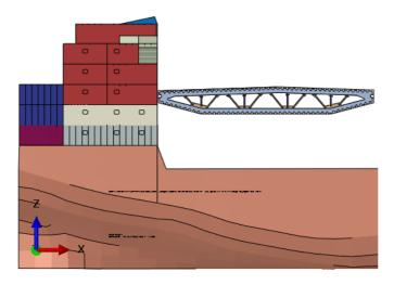
Figure 4-5 Deckhouse ship and bridge girder finite element model, impact between deck 2 and 3
