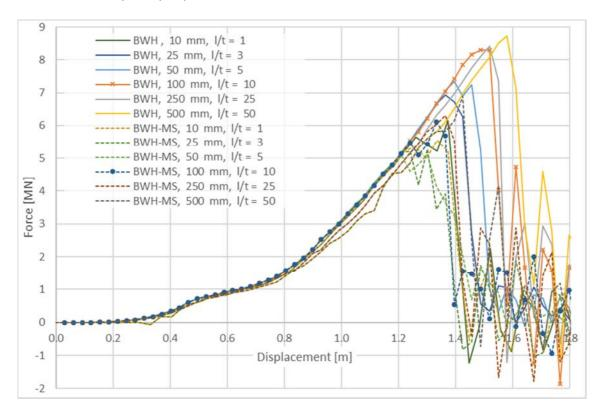
> Figure 3-7 Sensitivity study for BWH. MS – mesh scaling.
