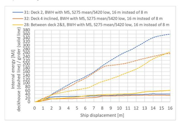
Figure 5-6 Internal energy [MJ] impact deckhouse-girder
