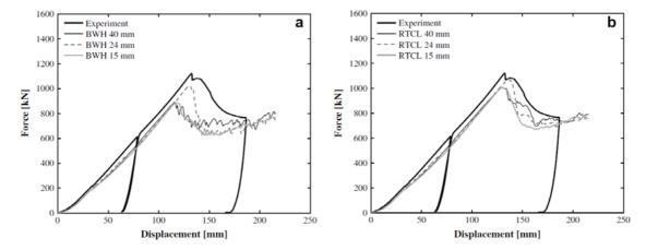
> Figure 3-3 Force-displacement behavior of panel 2-FB. Failure criterion scaling is used at the plate-stiffener junctions: (a) simulations using the BWH criterion, (b) simulations using the RTCL criterion [14]. Plate thickness 40 mm, 24 mm and 15 mm give a l/t-ratio of 8, 4.8 and 3 respectively.
