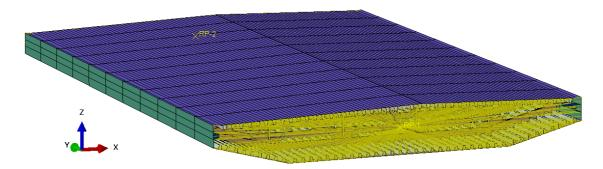
> Figure 4-11 Boundary condition at the cut-off boundary of the bridge girder
