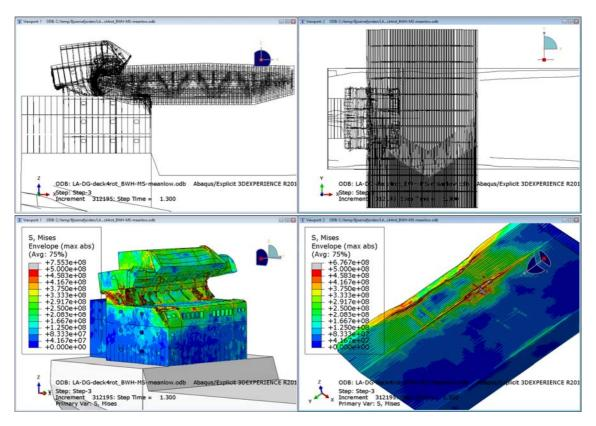
> Figure 5-3 von Mises stress [MPa] load case C: Bridge girder inclined at deck 4
