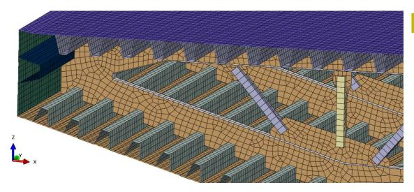
> Figure 4-10 Detailed mesh of the bridge girder
