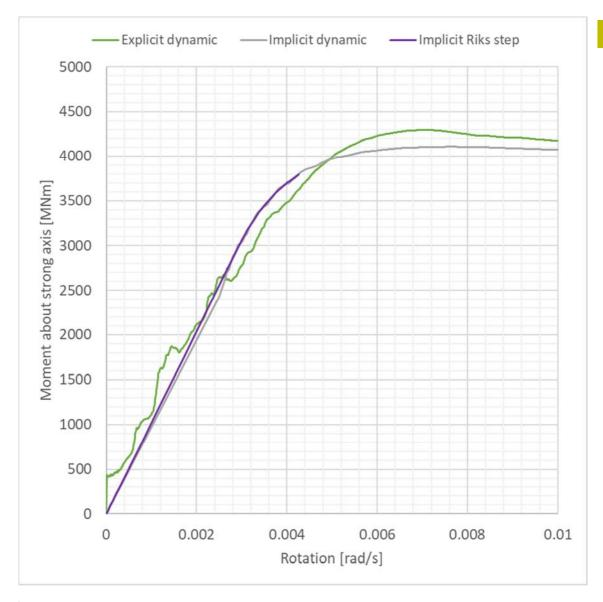
> Figure 5-15 Load-rotation curve for moment about strong axis for intact bridge girder, comparison with implicit analysis
