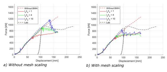
> Figure 3-4 Force-displacement curves for plate with two HP stiffeners from test and simulations with different mesh size. [9]
