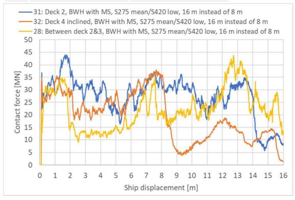
Figure 5-5 Contact force [MN] impact deckhouse-girder
