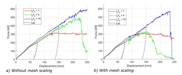
> Figure 3-5 Force-displacement curves for clamped plate with 6 L stiffeners from test and simulations with different mesh size. [9]
