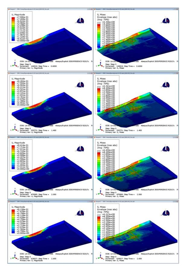
> Figure 5-10 Damaged bridge girder after approximately 4 m, 8 m, 12 m and 16 m ship displacement for impact at deck 2
