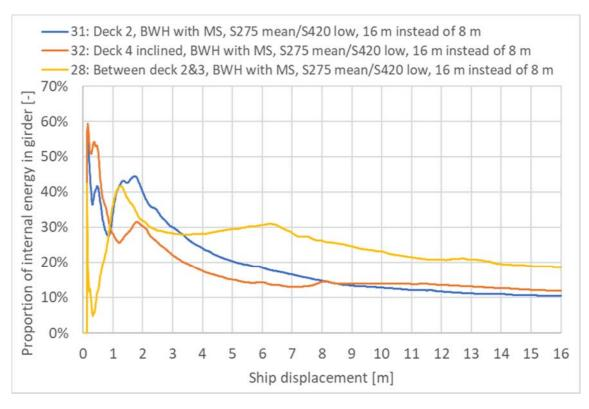
Figure 5-8 Proportion of internal energy in girder [-] impact deckhouse-girder
