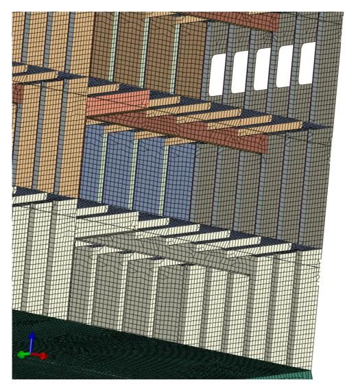
> Figure 4-9 Detailed mesh of the deckhouse ship
