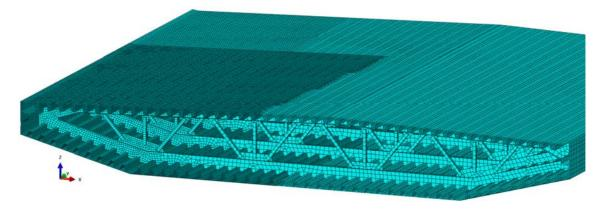
> Figure 4-8 Mesh of the bridge girder, shown cut in half
