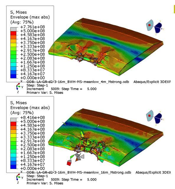
> Figure 5-11 Damaged bridge girder after 4 m (upper) and 16 m ship displacement (lower) applied with moment about strong axis. Deformations are scaled with factor 10 (and cause enlargement of damaged elements).
