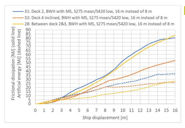
Figure 5-7 Frictional dissipation and artificial energy [MJ] impact deckhouse-girder
