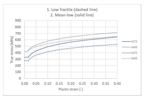
> Figure 4-6 True stress-strain curves of the steel materials, solid lines define the base case materials utilized
