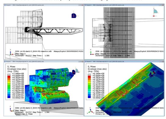
> Figure 5-4 von Mises stress [MPa] load case B: Bridge girder between deck 2 and 3
