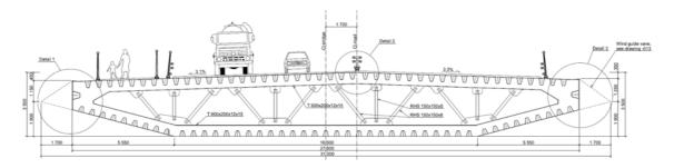
> Figure 4-1 Plan of the standard bridge girder cross section, from drawing K7-031 [18]
