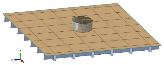
> Figure 3-6 Geometry of model for mesh sensitivity study
