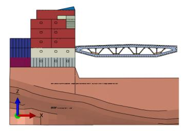
> Figure 4-3 Deckhouse ship and bridge girder finite element model, impact at deck 2
