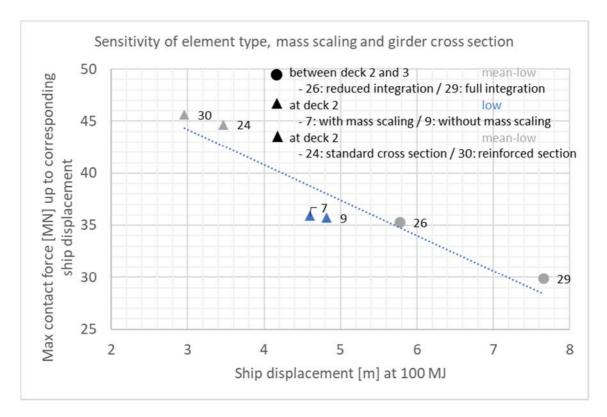
Figure 7-4 Sensitivity of element type, mass scaling and reinforced bridge girder cross section
