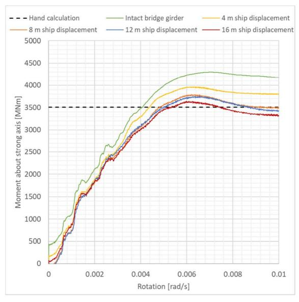
> Figure 5-13 Load-rotation curve for moment about strong axis
