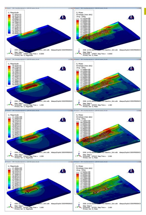
> Figure 5-9 Damaged bridge girder after approximately 4 m, 8 m, 12 m and 16 m ship displacement for impact between deck 2 and 3
