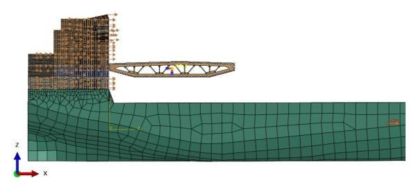
> Figure 4-13 Velocity applied to the deckhouse ship in step one
