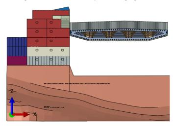
> Figure 4-4 Deckhouse ship and inclined bridge girder finite element model, impact at deck 4
