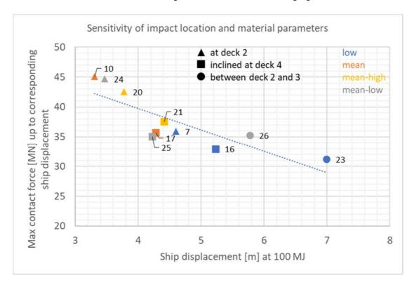
> Figure 7-2 Sensitivity of impact location and material parameters
