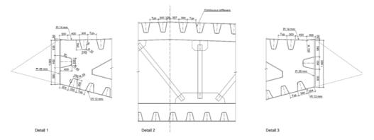
> Figure 4-2 Details of the standard cross section, from drawing K7-031 [18]
