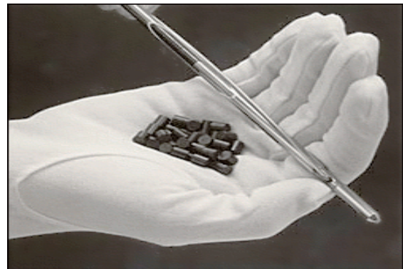
Figure 13.2: Fuel Pellets and Fuel Pellets Arranged in a Fuel Pin.
