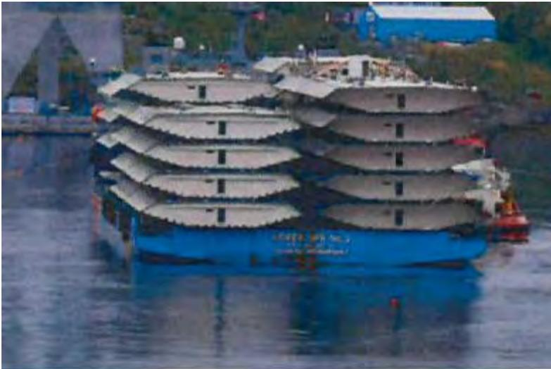
Figure 4-24 Barge used for Hålogaland
