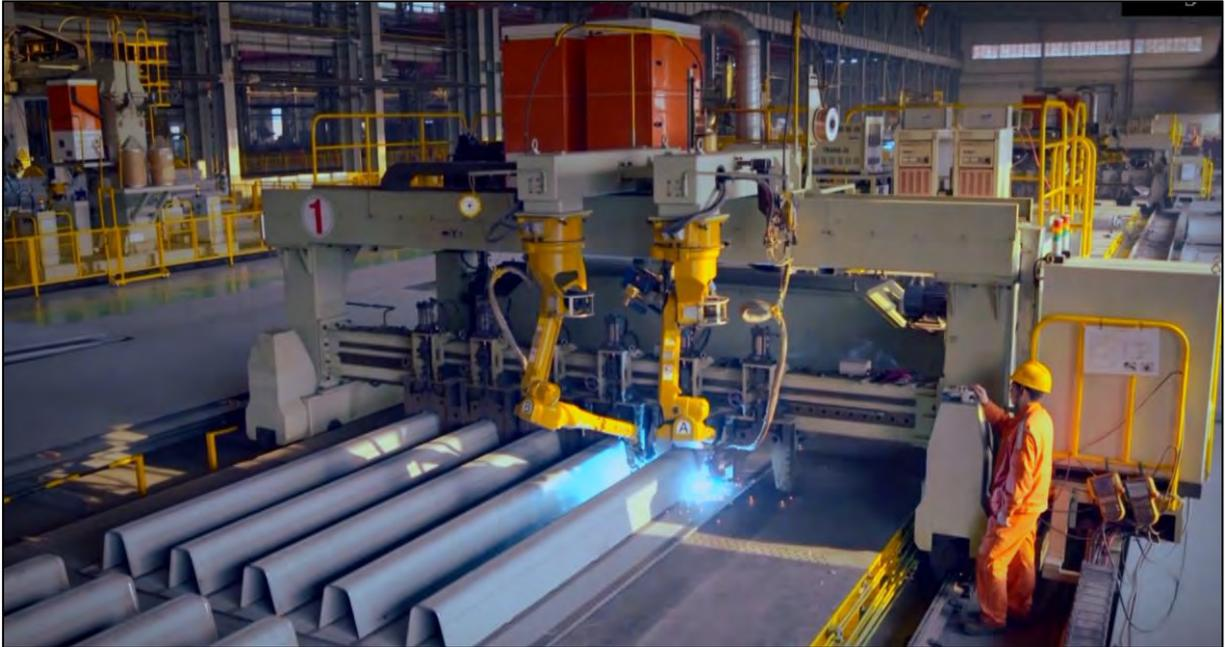
Figure 4-39 Robotic welding gantry in China. Process could be metal cored wire welding, or possibly MAG/CAW
