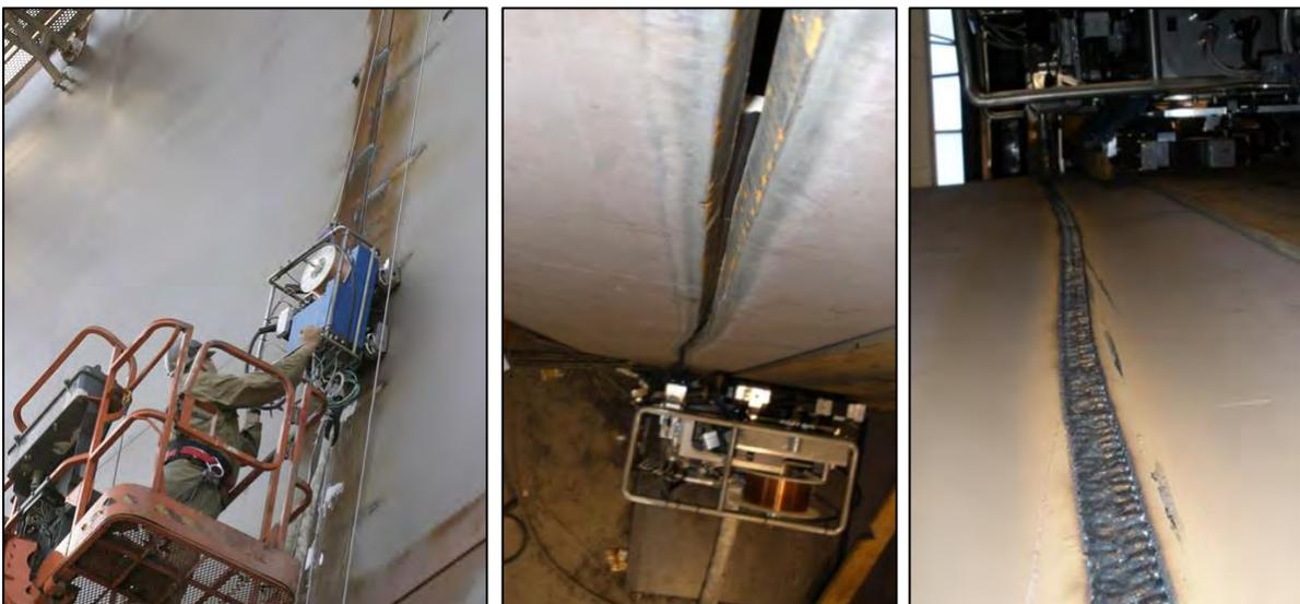
Figure 4-31 Self propelled and self positioning welding tractor for fully automated welding of section joints in the dock of OSS Lindø shipyard, using adaptive control to compensate for variations in groove position and gap
