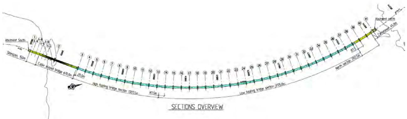
Figure 10-1: Overview of sections to be installed
