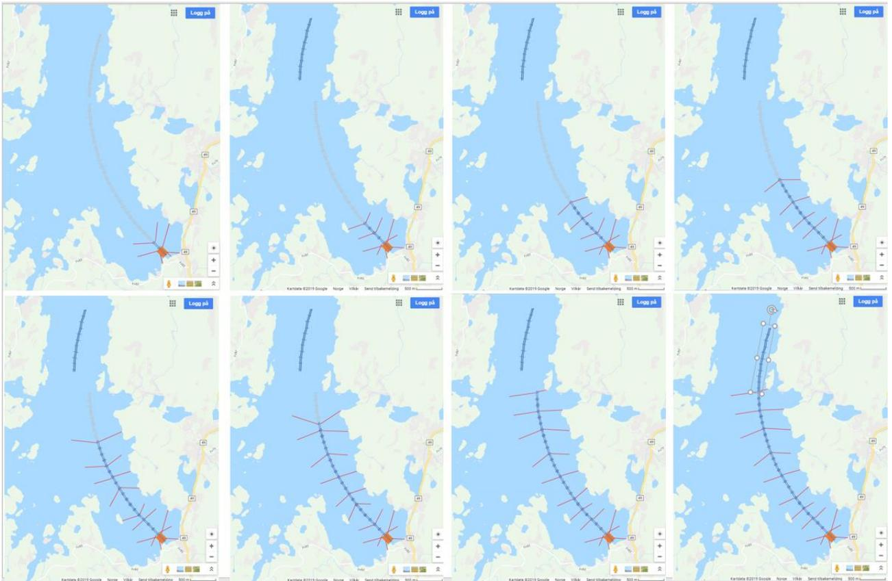
Figure 7-12: Low floating assembly and mooring process
