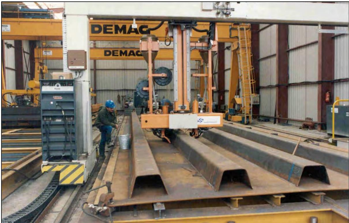
Figure 4-38 Gantry for welding on both sides of a trough simultaneously with submerged arc welding on the Pont de Normandie. Some gantries will now be able to weld all troughs on a panel in one take
