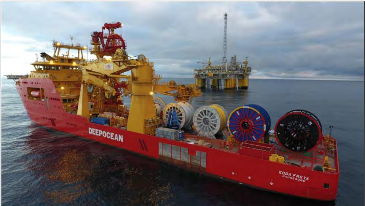
Figure 9-2: Edda Freya with 600t crane (©DeepOcean)
