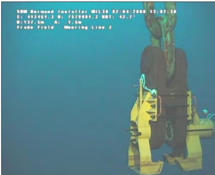
Figure 9-10 H-shackle with ROV-kit connected to bottom chain
