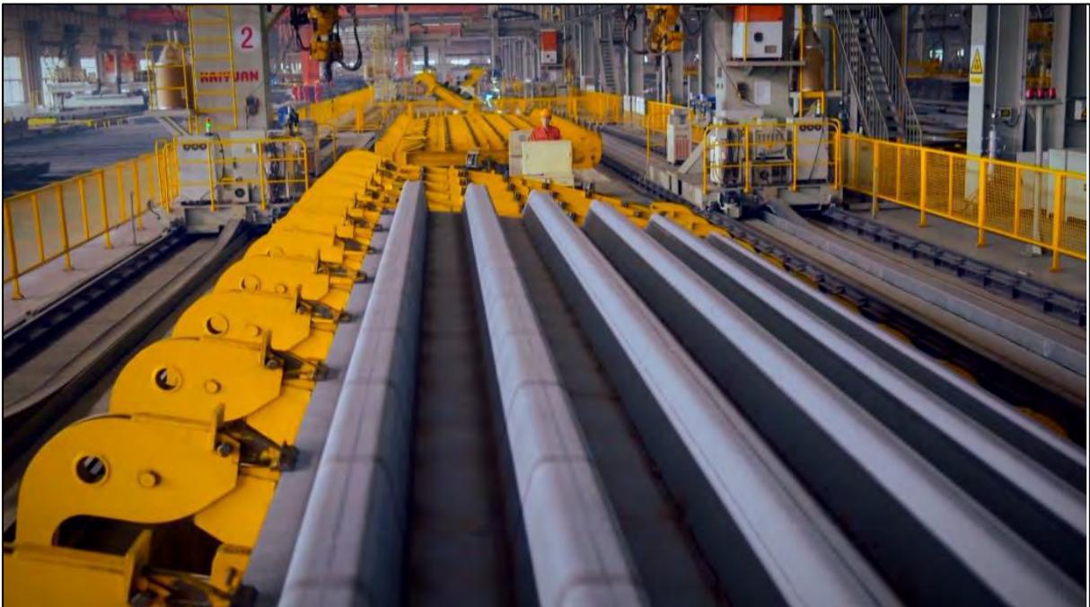
Figure 4-40 Deck panel with troughs on fixture, in China
