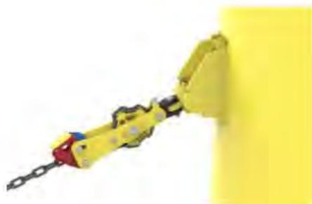
**Vessel Tensioned Mooring System**
