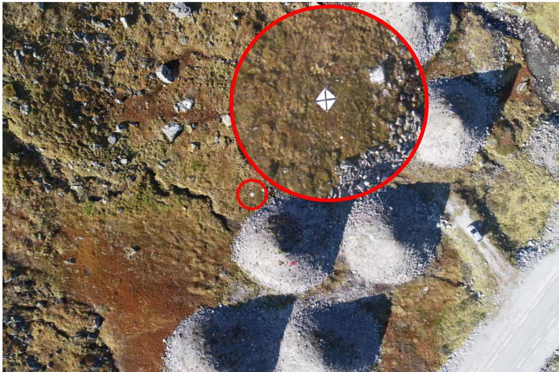
*Figure 2: Example of a photograph collected with the UAS, showing the avalanche braking mounds at the foot of the avalanche path on Sætreskarsfjellet; area encircled in red is enlarged (inset) to illustrate GCP placement in the scene.*
