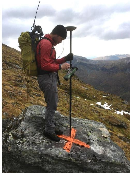
**Figure 4. Hallvard Nordbrøden (NPRA) surveying a ground control point at Storskreda, Lavangsdalen, during field work in October 2019. (Photo: Emil Solbakken)**
