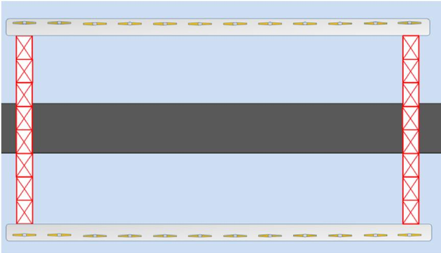
Figure 18 Concept for using truss structures and pontoons to allow for additional rows of TISEC devices in the downstream direction for a suspension bridge (seen from below).
