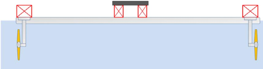
Figure 21 Concept for using truss structures to allow for additional rows of TISEC devices in the downstream direction for a floating bridge (seen from the side).
