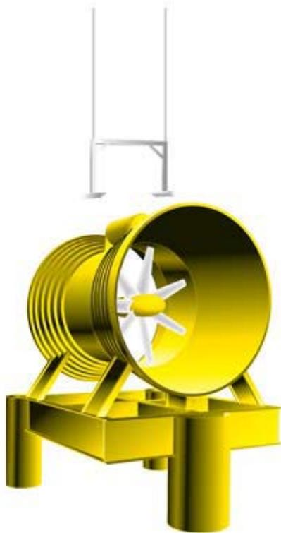
Figure 6 Enclosed tips (Venturi) design principle [19].
