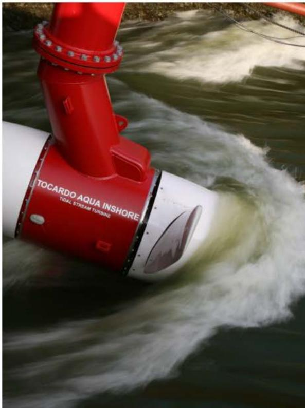
The Tocardo T100 system offers a complete water to grid solution for open flowing water like rivers, channels and tidal currents. The T100 has a rated output of 100 kW and is designed to operate at water speeds starting at 2 m/s (4 kts). The system is designed to minimize maintenance and maximize power output over its 20 year lifetime.
