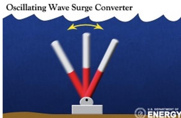
*Figure 10 Oscillating wave surge converter design principle [18].*
