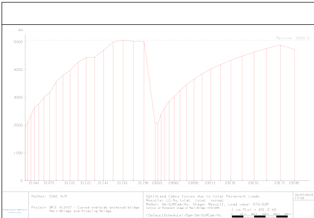
Figure 3-6: Cable forces measured on the jack – back and front stay cables.
