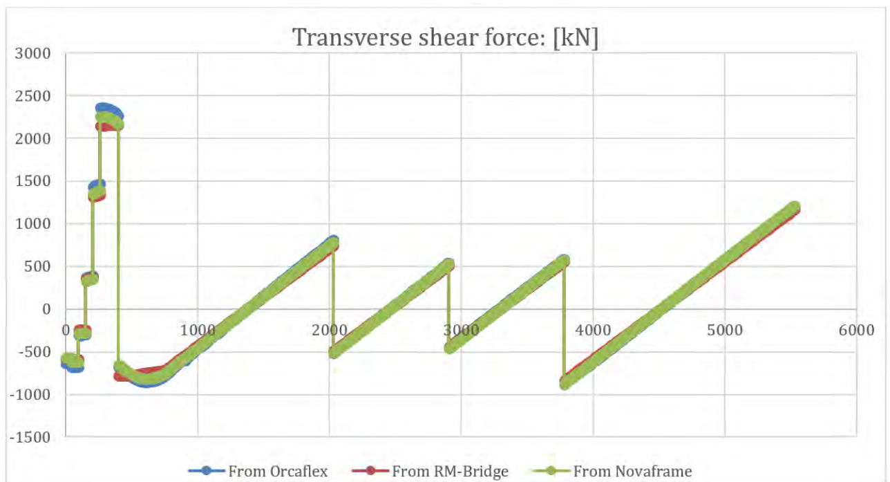
Figure 7-18 Comparison of transverse shear force for temperature load for K12 in kN
