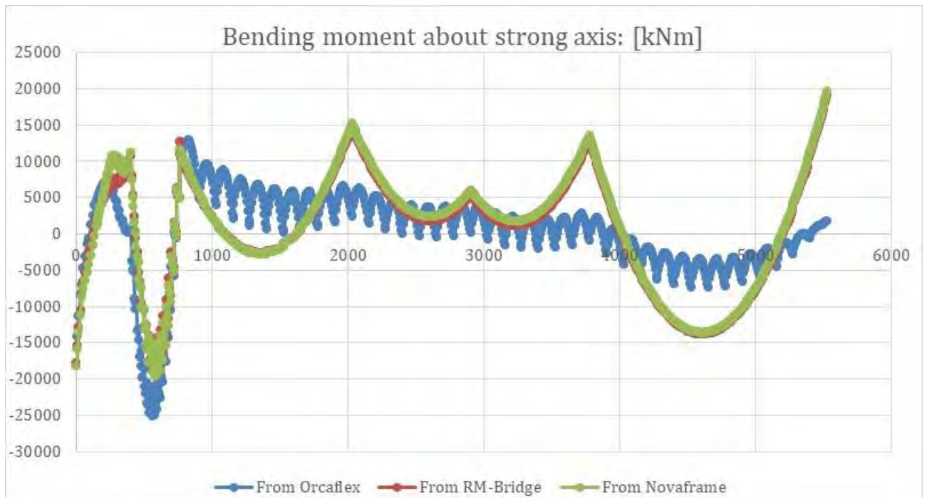
Figure 7-13 Bending moment about strong axis for torsional load for K12 in kNm
