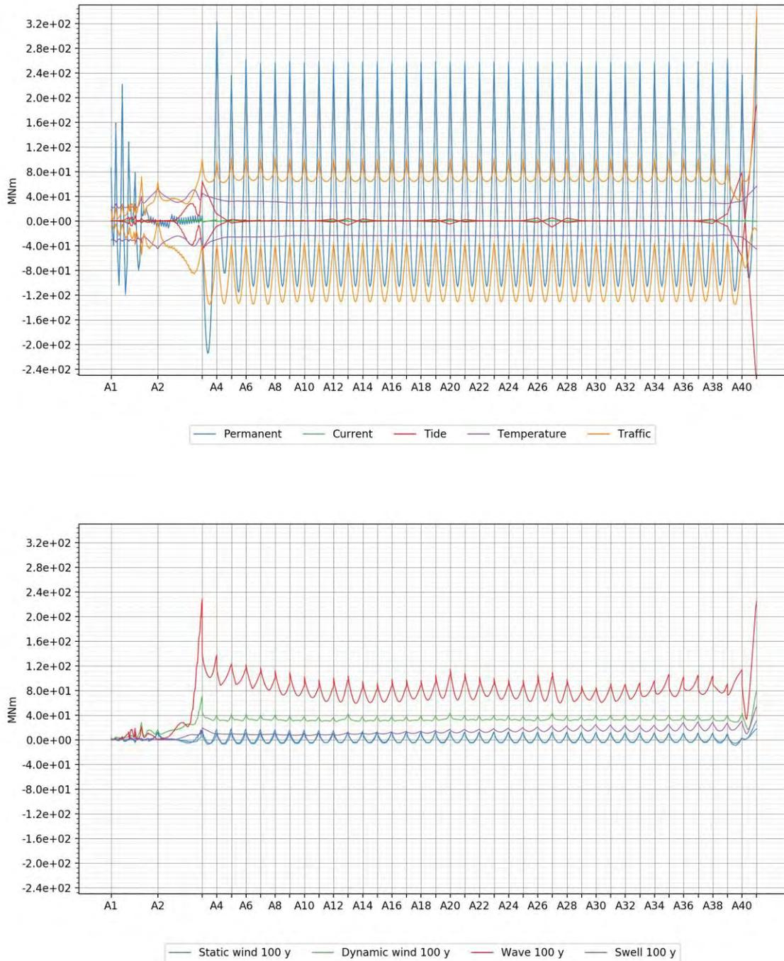
Figure 4-4 Overview of weak-axis bending moment contribution from slowly varying loads (top) and wave and wind loading (bottom) for the K12\_07 concept.
