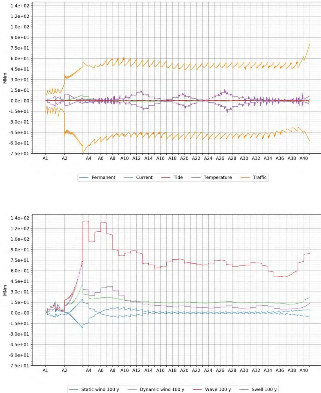
Figure 4-5 Overview of torsional moment contribution from slowly varying loads (top) and wave and wind loading (bottom) for the K12\_07 concept.
