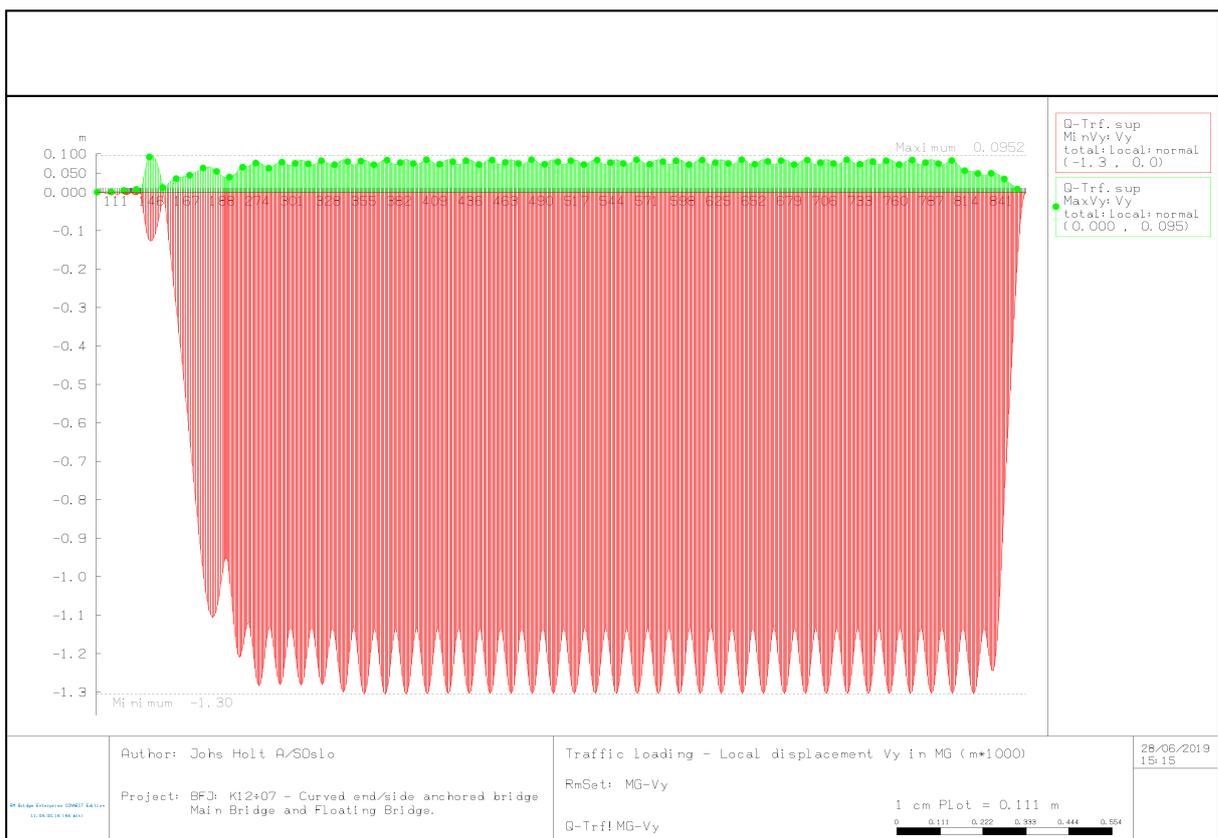
Figure 3-13 Traffic loading – vertical displacements in bridge girder (envelope values) [m]
