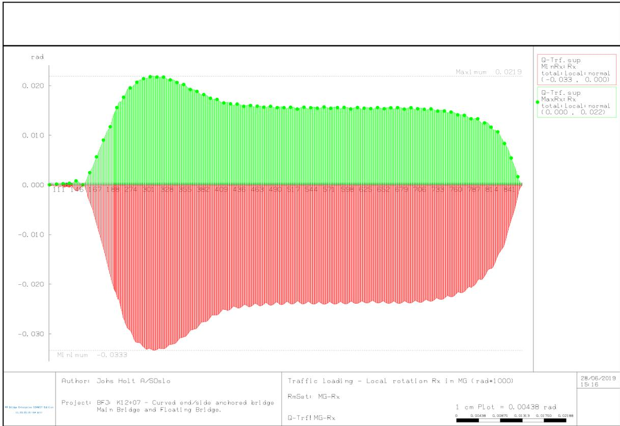
Figure 3-14 Traffic loading – rotation (roll) in bridge girder (envelope values) [rad]
