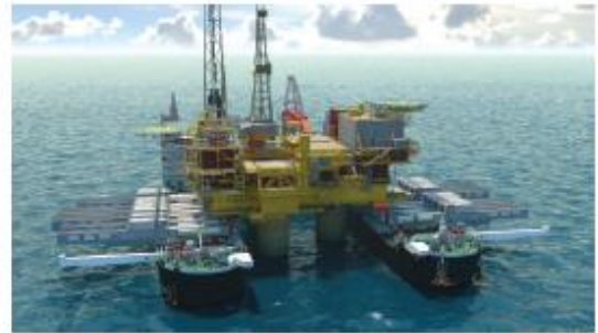
2. The vessel positions itself accurately to position the support yokes
