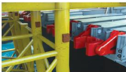
3. The active motion compensation system is engaged
