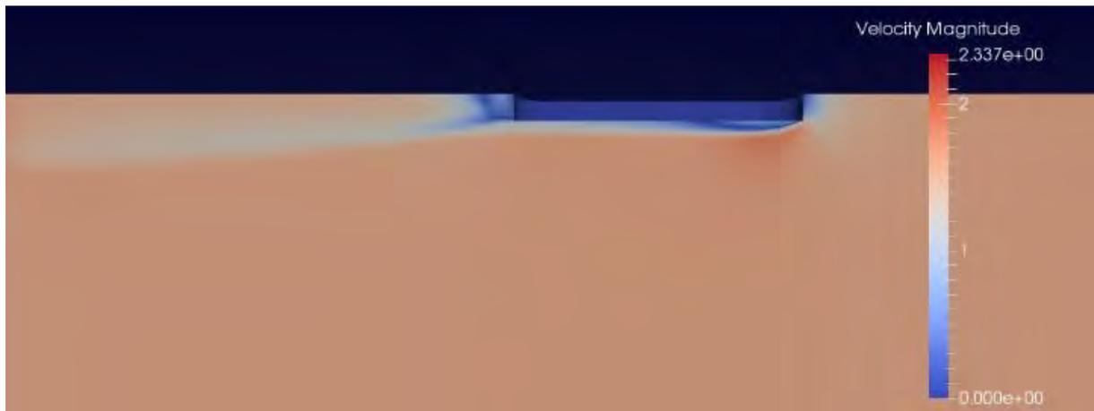
Figure 2-10 Velocity fields for pontoon in steady flow seen in a centre-cut parallel with the pontoons length axis.
