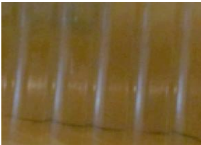
Figure 4-1 Inside of aged PA11 pressure sheath
