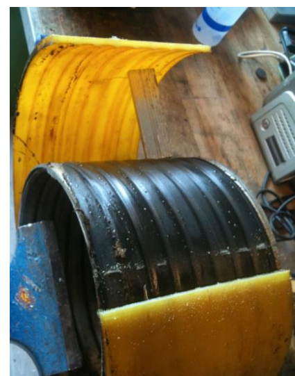
Figure 5-2 PA11 coupon extracted for analysis (Statoil), ref [28]
