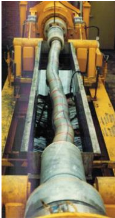
Figure 2-3 Rotating bending test of flexible riser, ref [12]
