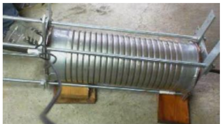
Figure 4-12 Testing of carcass radial leak rate (4Subsea)
