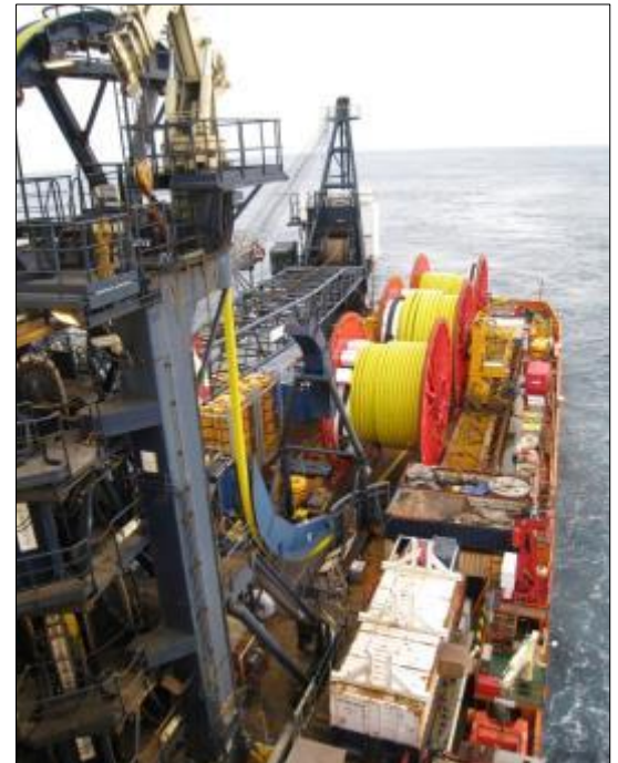
Figure 3-1 Flex riser replacement project (4subsea)
