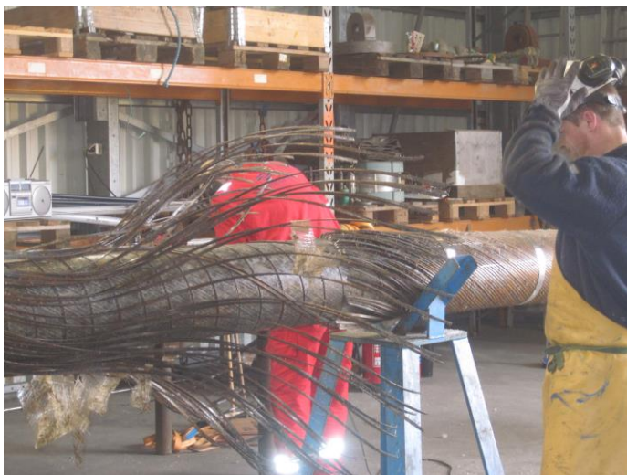
Figure 3-16 Removal of tensile armour wires for corrosion investigations (4Subsea)
