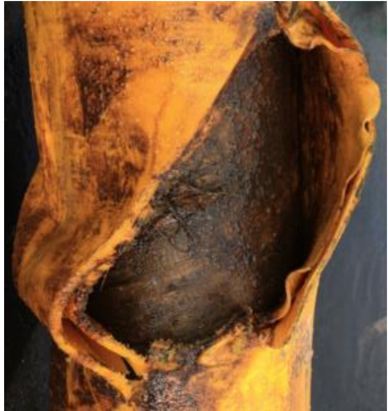
Figure 1-3 Typical external sheath failure due to pressure increase in the annulus, double external sheath (4subsea)
