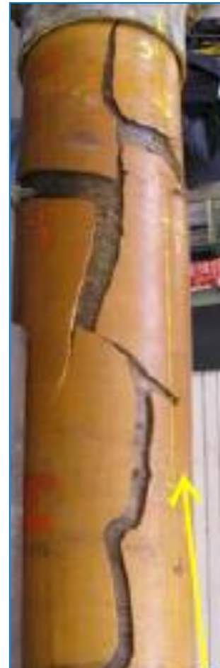
Figure 2-5 External sheath cracking due to high temperature under bending stiffer, ref [14]
