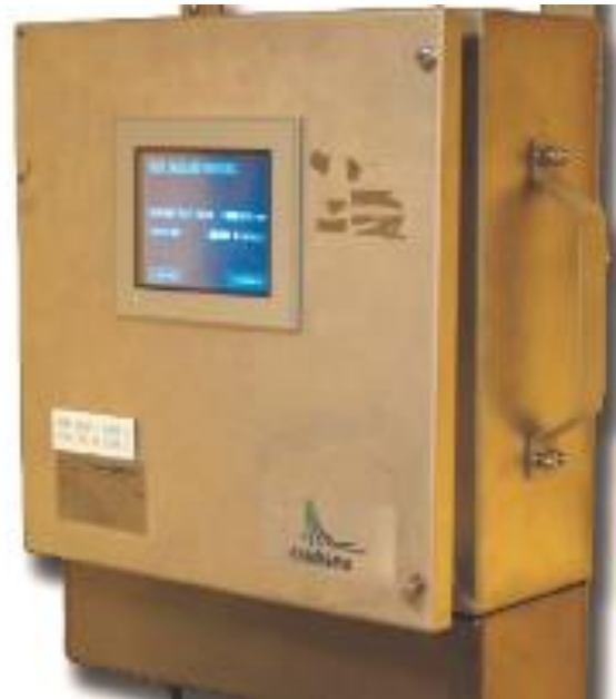
Figure 7-4 Typical online riser annulus vent monitoring cabinet (4Subsea)
