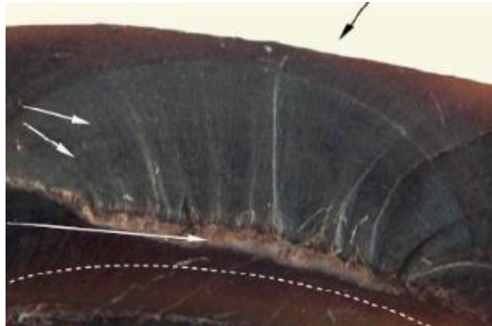
Figure 4-3 Fatigue growth in PVDF (secondary failure) after notch made by carcass failure (Talisman)
