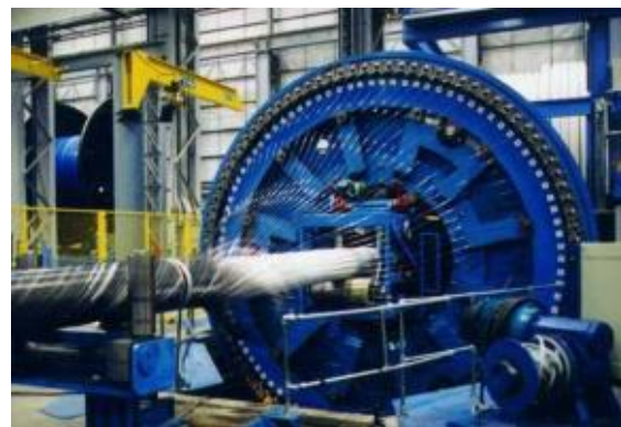
Typical armour wire winding station – Individual tensioned wires are carried on bobbins loaded on to the large rotating drum through which the pipe body is seen passing. The individual wires are lead onto the pipe body and spirally wound around it. The large drum may only rotate a few revolutions, making a few 10s of meters of pipe before it needs to be stopped so that a wire bobbin can be changed in order to stager wire welds so only one weld, or less, is included per wire pitch.
