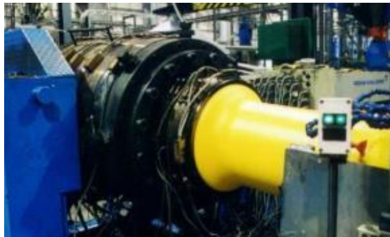
Typical extrusion of external sheath -- but similar to extrusion of a pressure sheath. The extrusion process for the inner and outer sealing layers has to be continuous because the melt process depends on friction in the extruder screw. If the flow of material is stopped, so is the melt process. Even after a few seconds of stoppage cooler material in the extruder disrupts the process.
